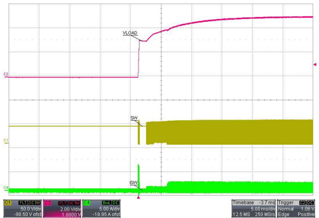
Figure 20. Short Circuit Recovery: V_{\text{SUPPLY}} = 36\text{V}
