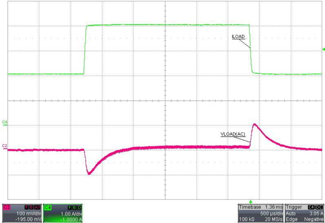
Figure 18. Load Transient, V_{\text{SUPPLY}} = 36\text{V} , I_{\text{LOAD}} = 2\text{A to } 4\text{A}
