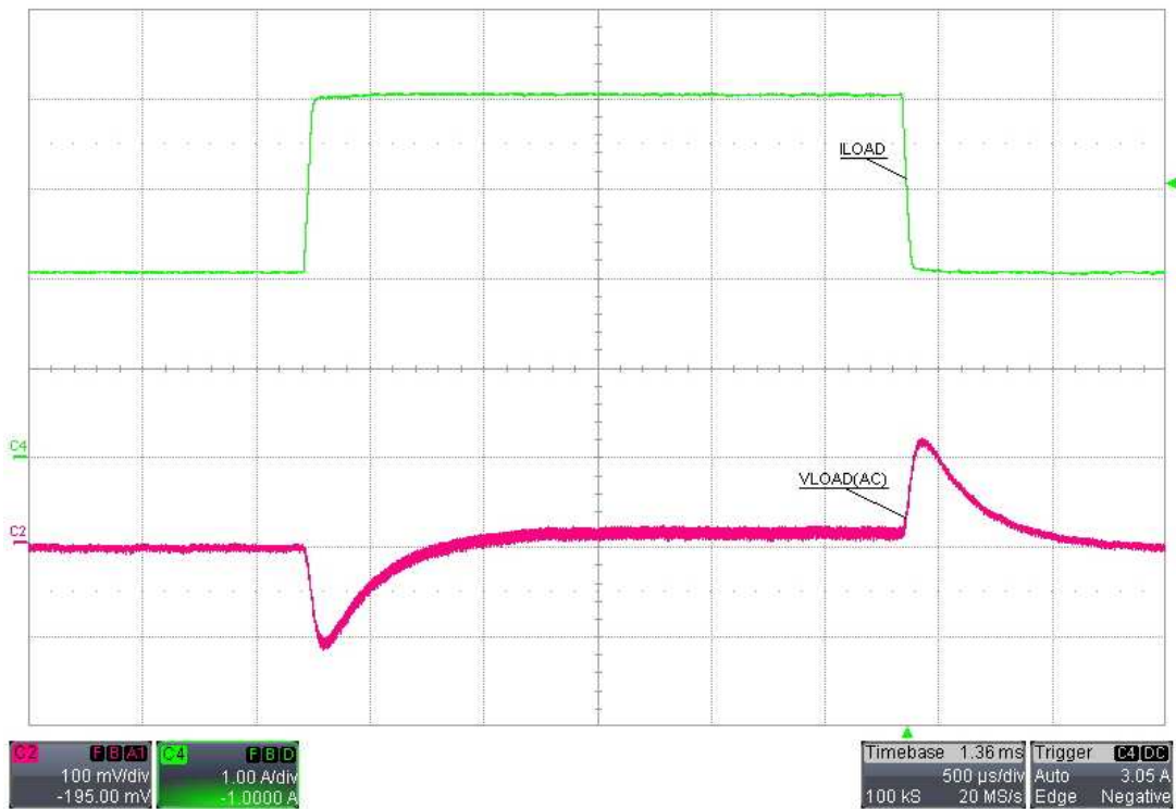
Figure 17. Load Transient, V_{\text{SUPPLY}} = 24\text{V} , I_{\text{LOAD}} = 2\text{A to } 4\text{A}
