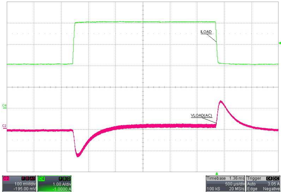
Figure 16. Load Transient, V_{\text{SUPPLY}} = 18\text{V} , I_{\text{LOAD}} = 2\text{A to } 4\text{A}
