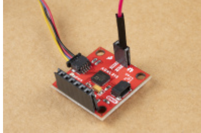
Close up of the wiring at the ADXL313 interrupt pin. (Click to enlarge)
