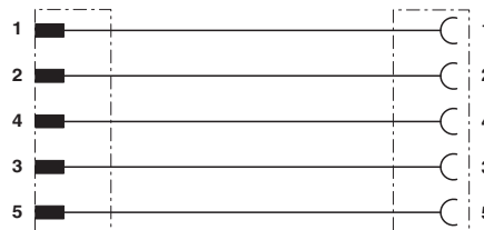
Contact assignment of the M12 plug and the M12 socket
