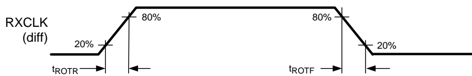
Figure 4. LVDS Output Transition Time
