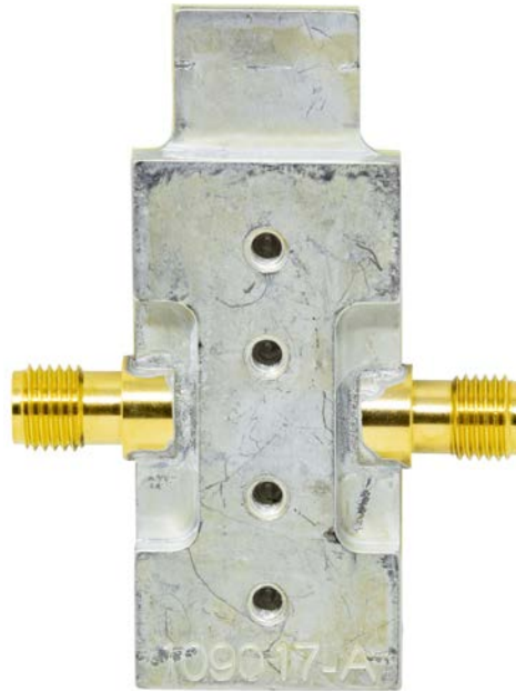
Figure 2. ADPA9002-EVALZ Secondary Side
