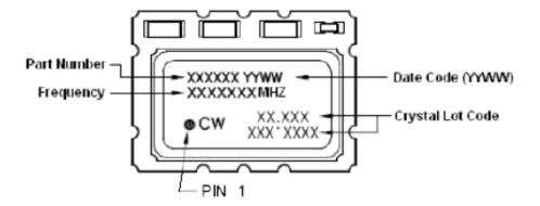
New configuration showing smaller crystal and 2-character (YM) date code format:
