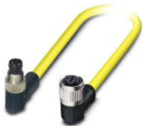
Sensor/actuator cable, 3-position, PVC, yellow, Plug angled M8, on Socket angled M12 SPEEDCON, A-coded, cable length: 0.5 m
