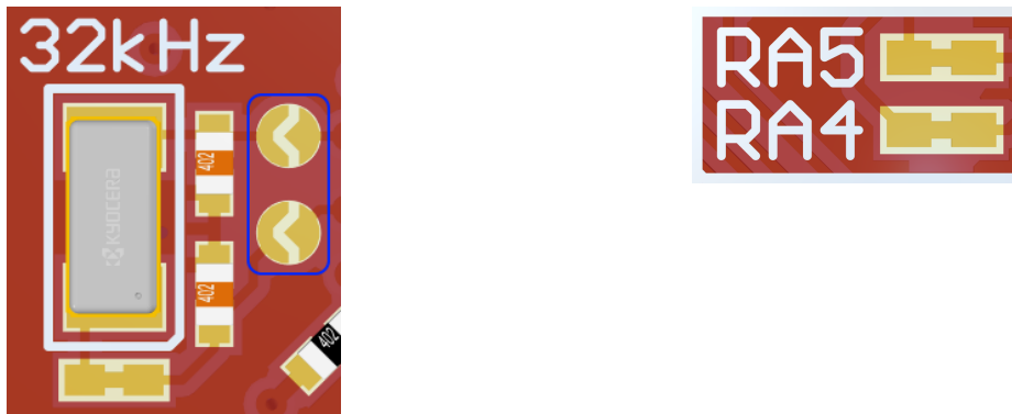
Figure 4-2. Crystal Connection and Cut Straps
