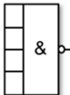
Figure 10-27 Logic gate with NAND operator
