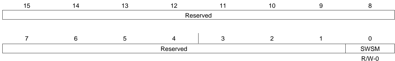
Figure 3-6. Software Wait-State Control Register (SWCR) [MMR Address 002Bh]
