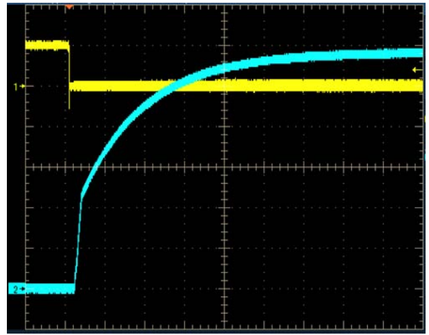
Fig.5: Turn-on transient at full rated load current (resistive) plus 5000uF at Vin=48V, triggered via ON/OFF pin. Top trace: ON/OFF signal (2V/div). Bottom trace: output voltage (5V/div). Time scale: 20ms/div
