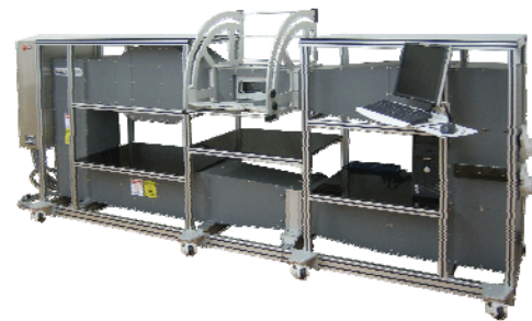
Fig. E: FDK Original Wind Tunnel
