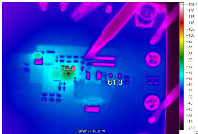
Figure 6. Thermal Performance V_{IN} = 48V , V_{OUT} = 12V , I_{OUT} = 20A , T_A = 23^{\circ}C , No Airflow
