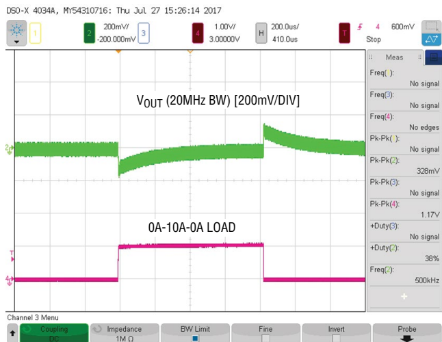
Figure 5. Load Step at V_{IN} = 48V , V_{OUT} = 12V
