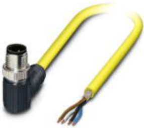
Sensor/actuator cable, 4-position, PVC, yellow, shielded, Plug angled M12 SPEEDCON, A-coded, on free cable end, cable length: 2 m
