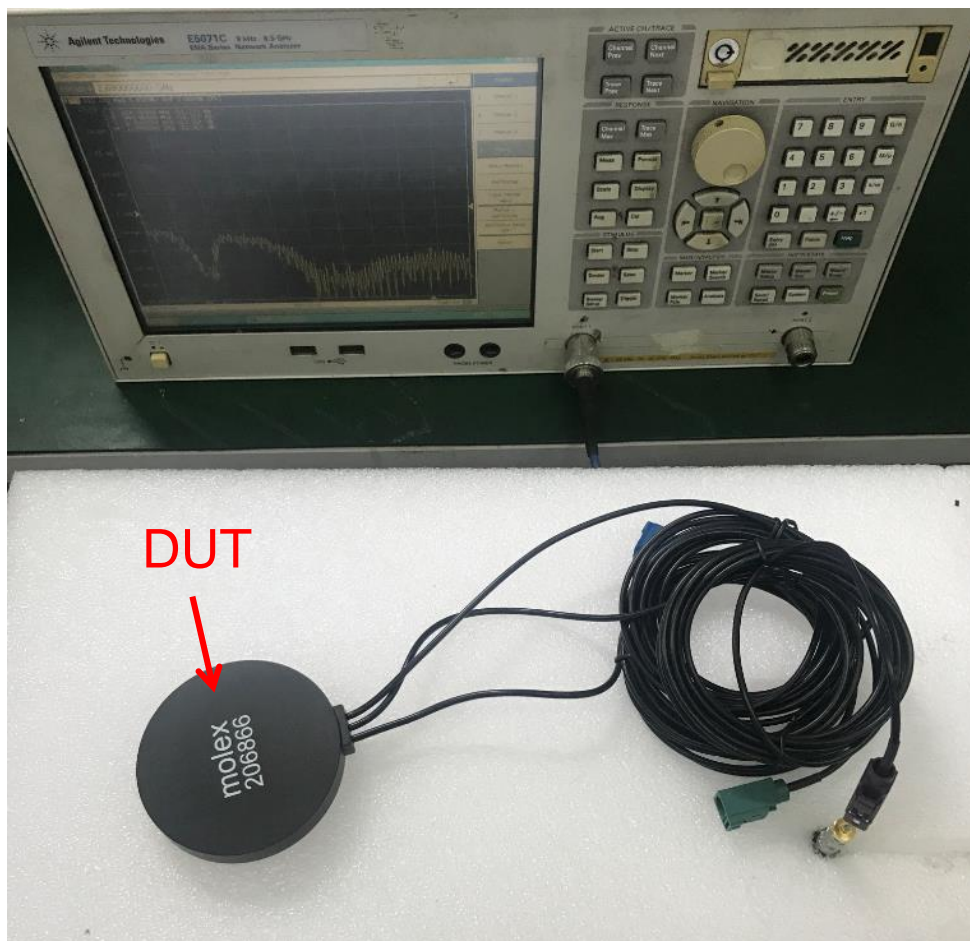
FIGURE 4.1.1 ANTENNA TESTED WITH VNA E5071C
