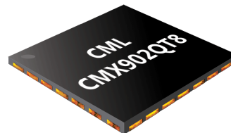
Small 28-pin WQFN Package (5mm x 5mm)
