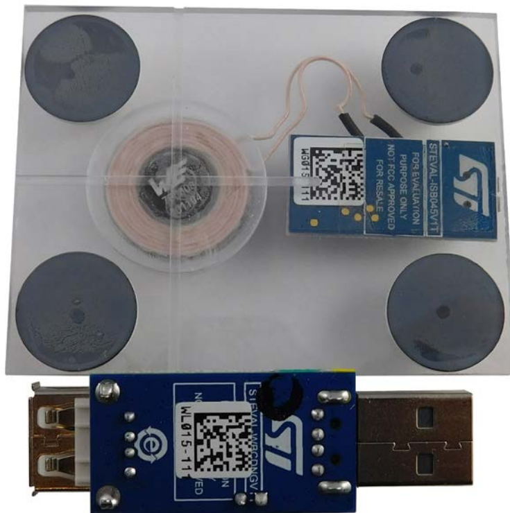
Figure 1. STEVAL-ISB045V1 evaluation kit
