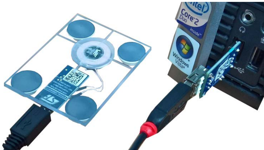
Figure 16. STEVAL-ISB045V1 evaluation kit connection
