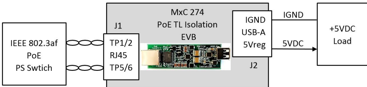
Figure 16: MxC 274 PoE Level 1 to USB-A +5Vreg Output TL EVB Block Diagram
