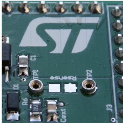
Figure 4. Mounting through-hole sense resistor
