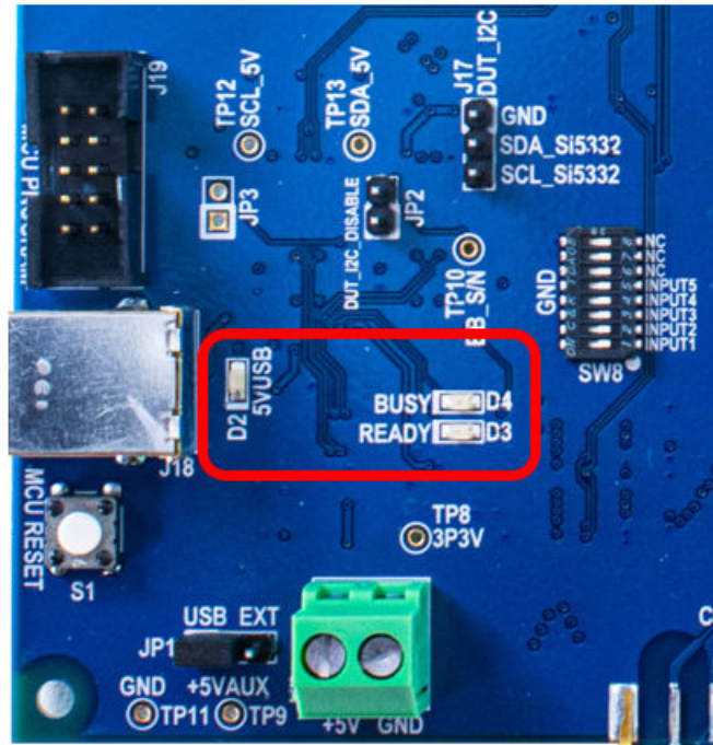
Figure 3.2. Si5332-6A-EVB LED Locations
