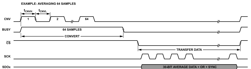
Figure 57. Example Conversion Cycle for Averaging Mode
