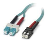
Assembled FO cable, zip cord cable, multi-mode fiberglass  $50/125 \, \mu m$ , OM3, plug: SC duplex/SC-RJ, degree of protection: IP20, for installation in cable ducts or control cabinets, length:  $2 \, m$
