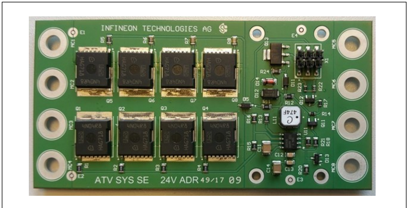
Figure 2 Battery Switch 24V - System Demonstrator Top View
