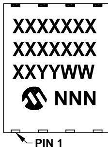
8-Lead DFN-S (6x5x0.9 mm)
