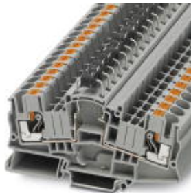
Component terminal block, with integrated P1000Y diode, connection method: Push-in connection, cross section: 0.5 mm 2 - 10 mm 2 , AWG: 20 - 10, width: 8.2 mm, color: gray
