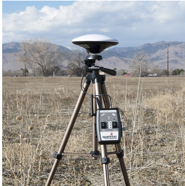
Temporary RTK Surveyor Base setup
