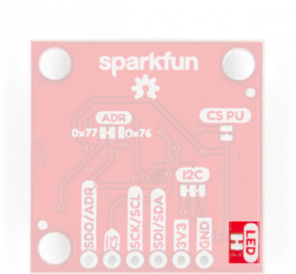
Annotated image of LED jumper. (Click to enlarge)
