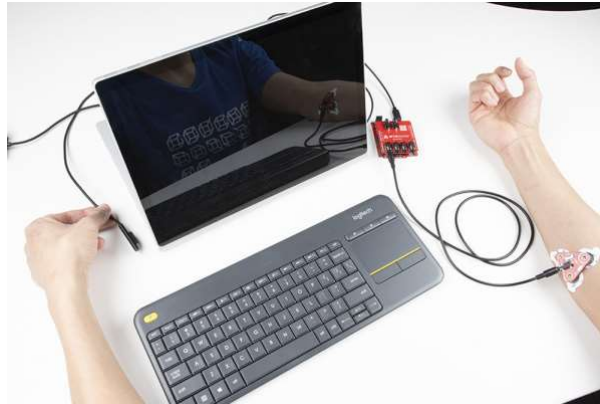
Removing power from a laptop before connecting the MyoWare.
