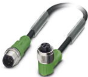
Sensor/actuator cable, 3-position, PUR halogen-free, black-gray RAL 7021, Plug straight M12, A-coded, on Socket angled M12, A-coded, cable length: 1.5 m
