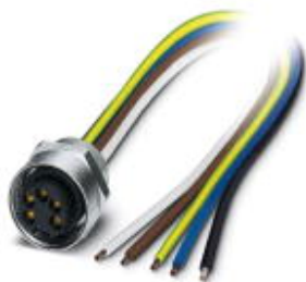
Sensor/actuator flush-type socket, 5-pos., 7/8", front mounting with Pg13.5 thread, with 0.5 m PVC litz wire, 5 x 0.75 mm 2
