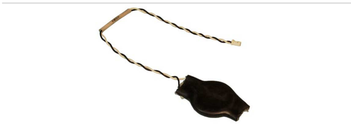
Figure 16. VL-CBR-0203 Latching Battery Module
