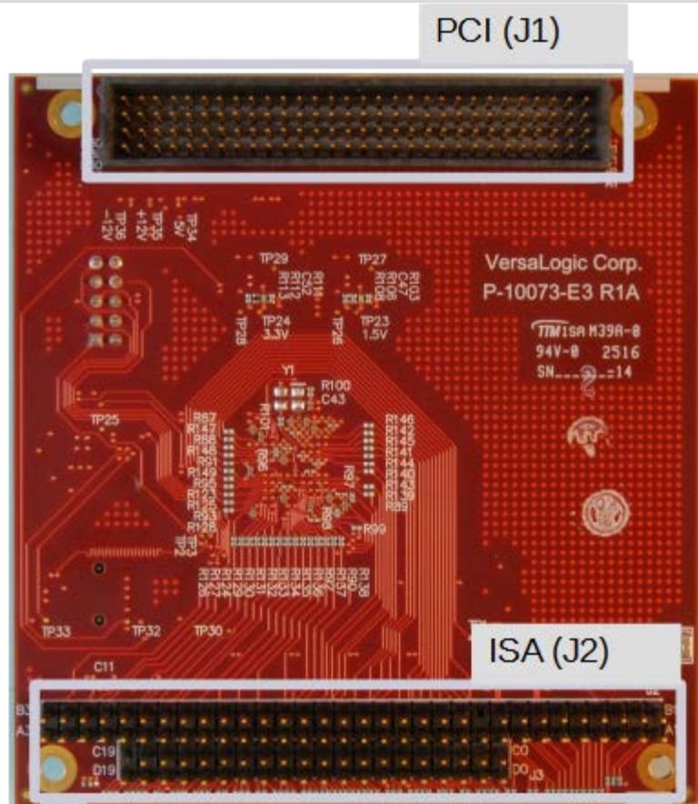
Figure 2. Major Components and Connectors (Bottom Side)
