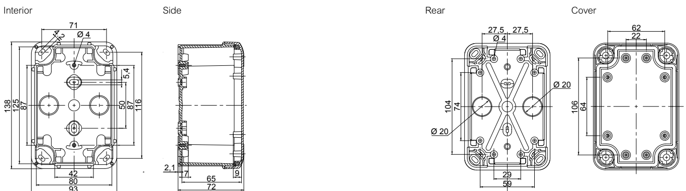
Box of 138 (5.43) x 93 (3.66) x 72 mm (in.) (external dimensions) NSYTB●●●1397
