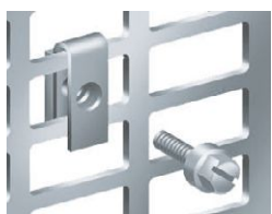
Direct mounting of equipment on nuts.
