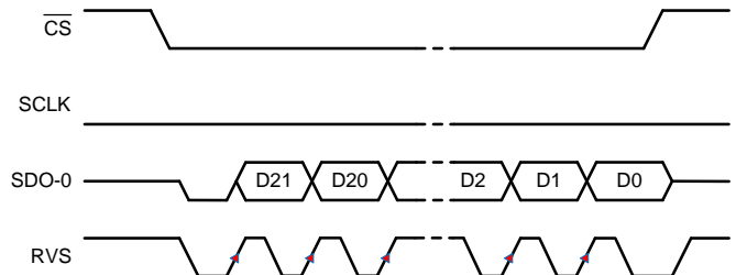
Figure 76. SRC-INT-SS: SRC, INTCLK, Single SDO, SDR
