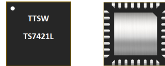
Figure 1 Device Image (32 Pin 4x4x0.8mm QFN Package)
