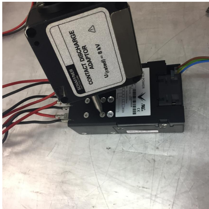
Figure 7: ESD Test Set up
