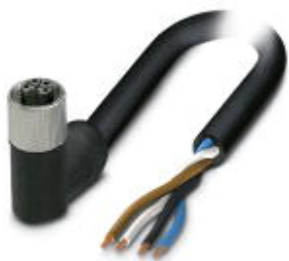
Power cable, 4-position, PVC, black-gray RAL 7021, Socket angled M12, L-coded, on free cable end, cable length: 1.5 m, for direct current up to 16 A/63 V
