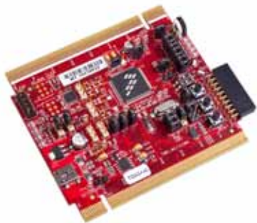
Figure 3: TWR-MCF51MM with Default Jumpers Used in Table 1
