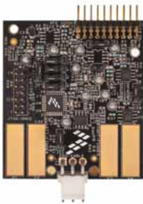
Figure 4: MED-EKG with Default Jumpers Used in Table 2
