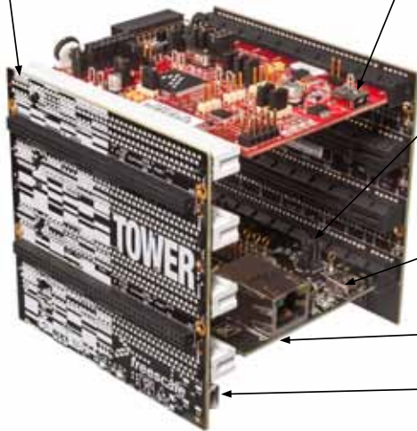
Figure 2: Tower System Assembled
