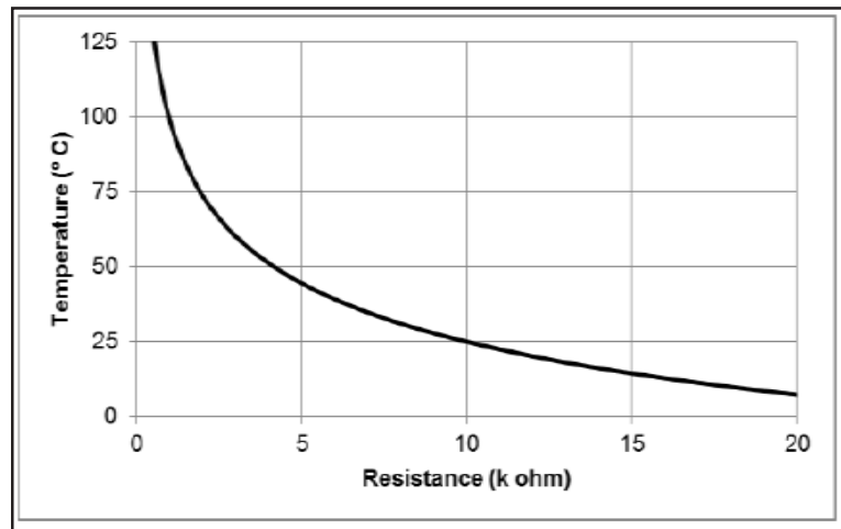
Figure 13: Coreboard temperature as a function of thermistor resistance
