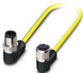
Sensor/actuator cable, 4-position, PVC, yellow, Plug angled M12 SPEEDCON, A-coded, on Socket angled M12 SPEEDCON, A-coded, cable length: 3 m
