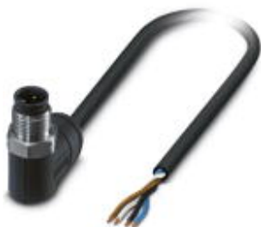
Sensor/actuator cable, 4-position, PE-X halogen-free, black-gray RAL 7021, Plug angled M12, A-coded, on free cable end, cable length: 5 m, for outdoor applications, with high-grade steel knurl
