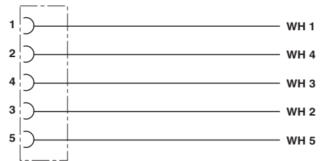
Contact assignment of the M12 socket
