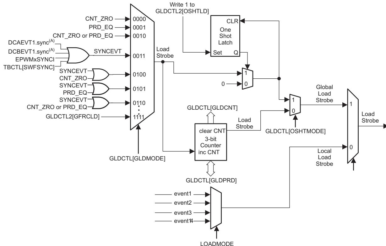
**NOTE:** The SYNC EVT signal is only propagated through when PHSEN is SET.
