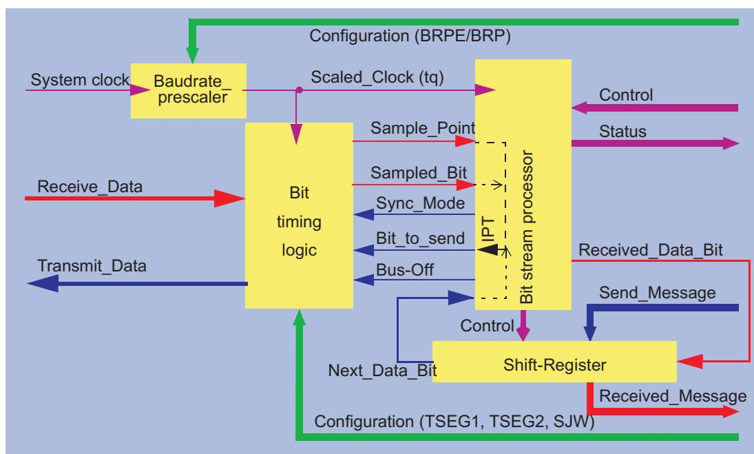
In this bit timing register, the components TSEG1, TSEG2, SJW and BRP have to be programmed to a numerical value that is one less than its functional value; so instead of values in the range of [1...n], values in the range of [0...n-1] are programmed. That way, for example, SJW (functional range of [1...4]) is represented by only two bits.
