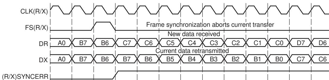
In contrast with [Figure 20-43](#), [Figure 20-44](#) shows McBSP operation when unexpected frame-synchronization signals are ignored (when (R/X)FIG = 1). Here, the transfer of word B is not affected by an unexpected pulse.
