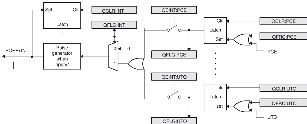
Eleven interrupt events (PCE, PHE, QDC, WTO, PCU, PCO, PCR, PCM, SEL, IEL and UTO) can be generated. The interrupt control register (QEINT) is used to enable/disable individual interrupt event sources. The interrupt flag register (QFLG) indicates if any interrupt event has been latched and contains the global interrupt flag bit (INT).
