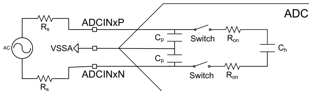
These input models should be used along with actual signal source impedance to determine the acquisition window duration. See [Section 10.15.2](#) for more information.
