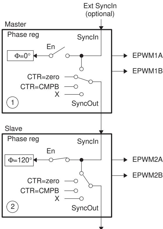
The following figure shows the associated timing waveforms for this configuration. Here, TBPRD = 600 for both master and slave. For the slave, TBPHS = 200 (that is,  $200/600 \times 360^\circ = 120^\circ$ ). Whenever the master generates a SyncIn pulse (CTR = PRD), the value of TBPHS = 200 is loaded into the slave TBCTR register so the slave time-base is always leading the master's time-base by 120°.
