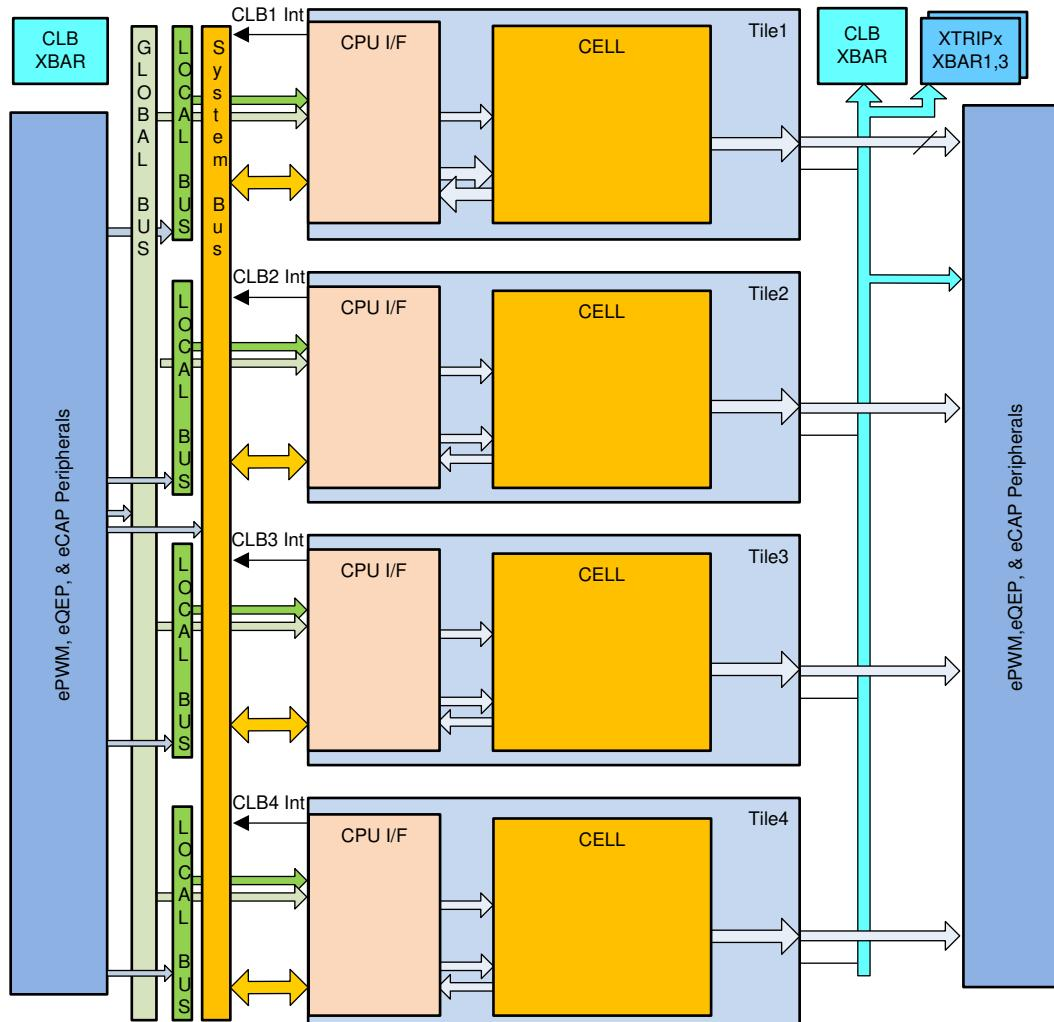
The tile contains the core logic, providing the logic reconfiguration capability. Each CLB tile is associated with a separate CPU interface, which contains the registers needed to control and configure the logic in the tile. The CPU interface also contains data transfer buffers that can be used as part of the configurable logic to exchange data with the rest of the device. [Figure 25-2](#) shows the connections between the tile, the CPU interface, and the device.
