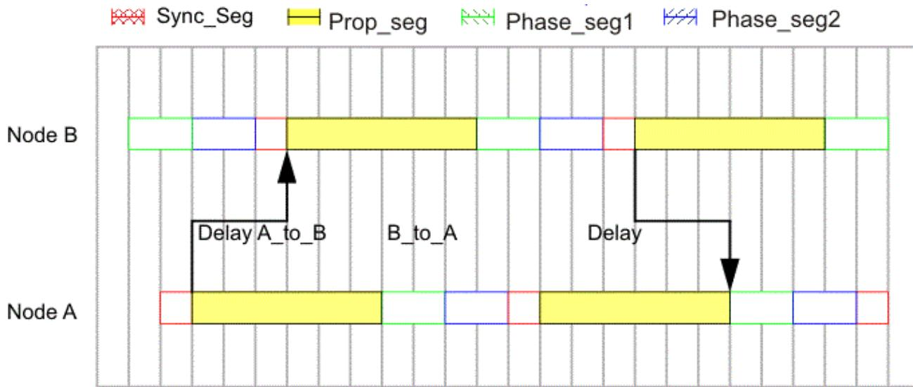
$$\text{Delay A\_to\_B} \geq \text{node output delay(A)} + \text{bus line delay (A-B)} + \text{node input delay(B)}$$
