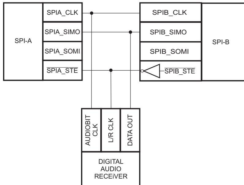
Standard C28x SPI timing requirements limit the number of digital audio interface formats supported using the 2-SPI configuration with the STEINV bit. See your device-specific data sheet electrical specifications for SPI timing requirements. With the SPI clock phase configured such that the CLKPOLARITY bit is 0 and the CLK\_PHASE bit is 1 (data latched on rising edge of clock), standard right-justified digital audio interface data format is supported as shown in [Figure 17-13](#).
