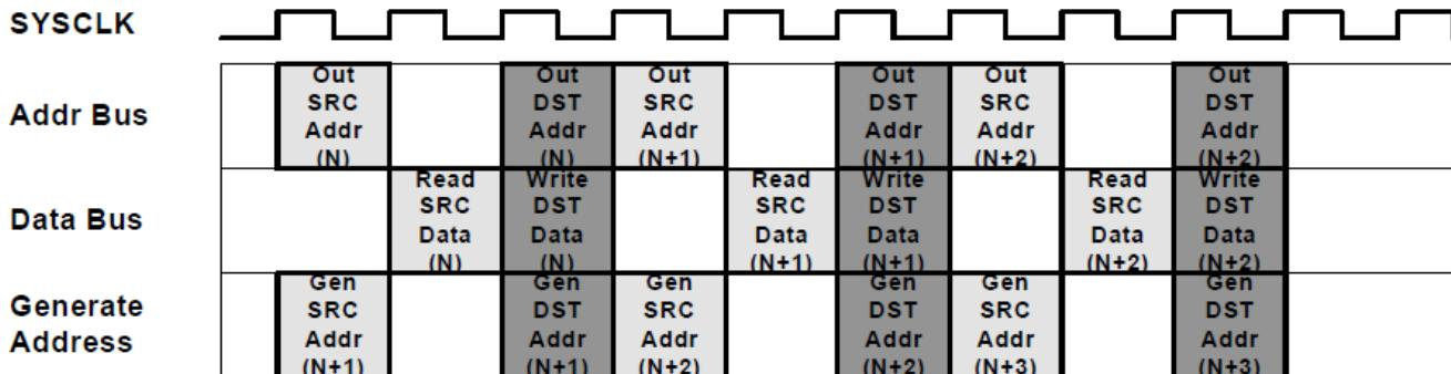
**Figure 5-7. 3-stage Pipeline With One Read Stall**
