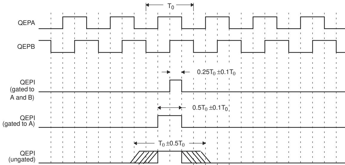
Some typical applications of shaft encoders include robotics and computer input in the form of a mouse. Inside your mouse you can see where the mouse ball spins a pair of axles (a left/right, and an up/down axle). These axles are connected to optical shaft encoders that effectively tell the computer how fast and in what direction the mouse is moving.
