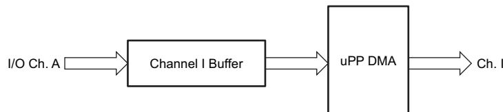
[Figure 23-4](#) explains the data flow for receive in DDR demux mode. In this case, both DMA channels (channel I and channel Q) are used.
