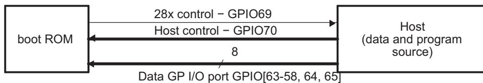
The control subsystem communicates with the external host device by polling/driving the GPIO70 and GPIO69 lines. The handshake protocol shown in [Figure 4-14](#) must be used to successfully transfer each word via GPIO [63-58,64,65]. This protocol is very robust and allows for a slower or faster host to communicate with the master subsystem.
