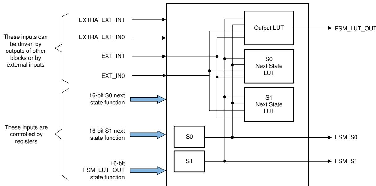
The signals and functionality of the FSM block are described below:
