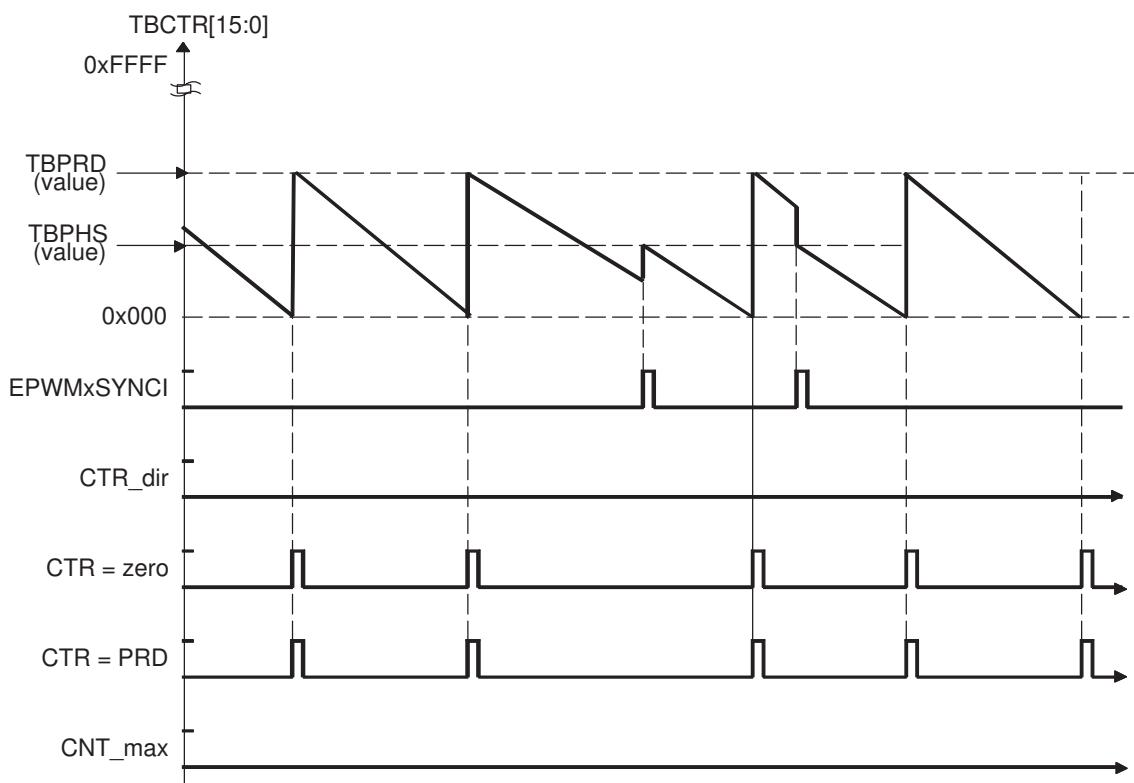
**Figure 14-10. Time-Base Up-Down-Count Waveforms, TBCTL[PHSDIR = 0] Count Down On Synchronization Event**
