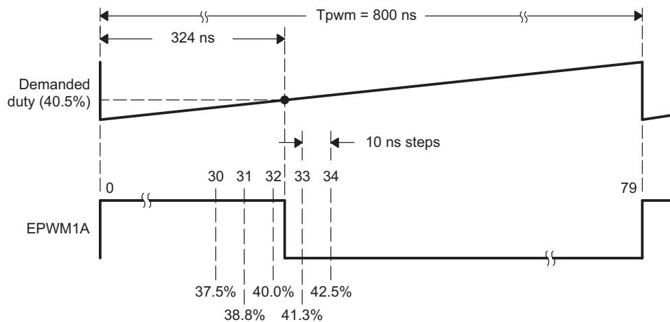
**Table 14-15. CMPA vs Duty (left), and [CMPA:CMPAHR] vs Duty (right)**
