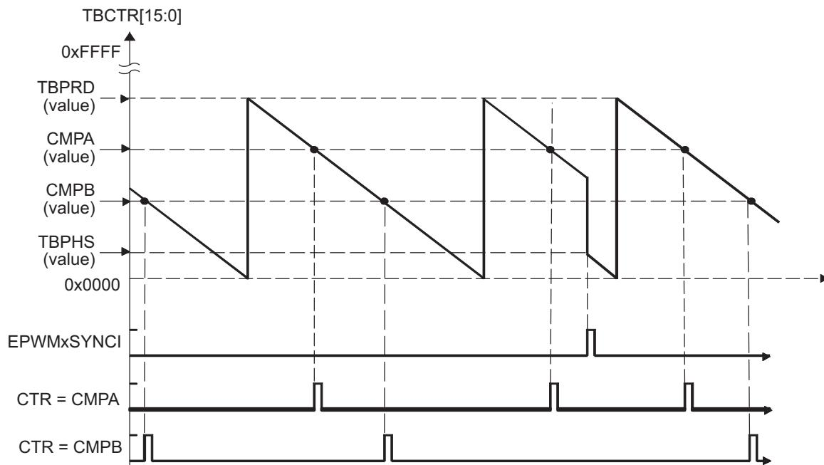
**Figure 14-17. Counter-Compare Events In Up-Down-Count Mode, TBCTL[PHSDIR = 0] Count Down On Synchronization Event**
