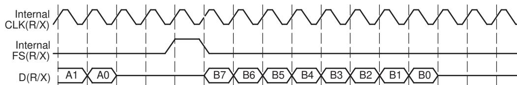
**NOTE:** The McBSP cannot operate at a frequency faster than  $\frac{1}{2}$  the LSPCLK frequency. When driving CLKX or CLKR at the pin, choose an appropriate input clock frequency. When using the internal sample rate generator for CLKX and/or CLKR, choose an appropriate input clock frequency and divide down value (CLKDV) (that is, be certain that CLKX or CLKR  $\leq$  LSPCLK/2).
