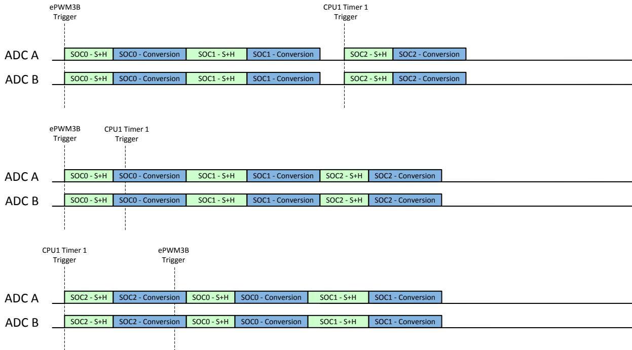
Note that any trigger source that can be selected in the TRIGSEL field can be used except for software triggering. There is no way to issue the software triggers for all ADCs simultaneously, so it will likely result in asynchronous operation. ADCINT1 or ADCINT2 can also be used as a trigger as long as the ADCINTSOCSEL1 and ADCINTSOCSEL2 registers are configured identically for all ADCs and software triggering is not used to start the chain of conversions.
