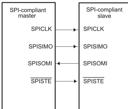
The master device controls the flow of communication by providing shift-clock and slave-enable signals. The slave-enable signal is an optional active-low signal that enables the serial data input and output of the slave device (device not sending out the clock).
