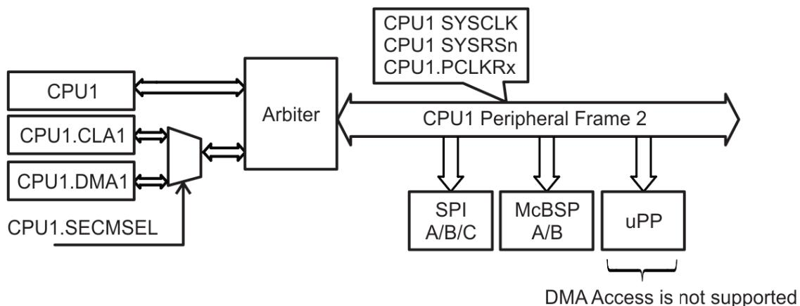
**NOTE:** If CPU and DMA make an access to the same peripheral frame in the same cycle, the DMA has priority and the CPU is stalled.
