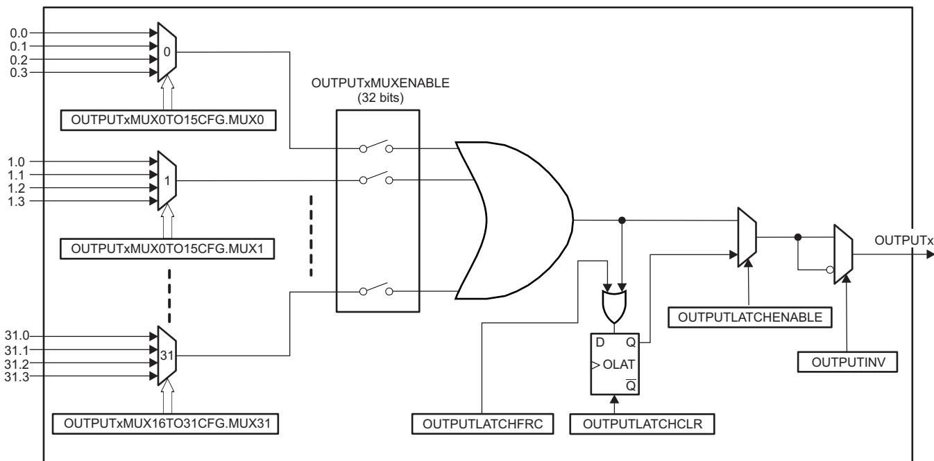
First, determine the signal(s) which should be passed to the GPIO by referencing [Table 8-4](#). You may select up to one signal per mux (32 total muxes) for each OUTPUTXBARx output. Select the inputs to each mux via the OUTPUTxMUX0TO15CFG and OUTPUTxMUX16TO31CFG registers.
