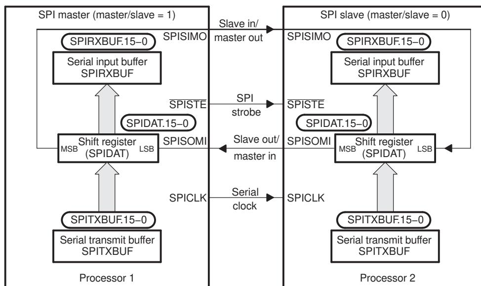
The SPI can operate in master or slave mode. The MASTER\_SLAVE bit selects the operating mode and the source of the SPICLK signal.
