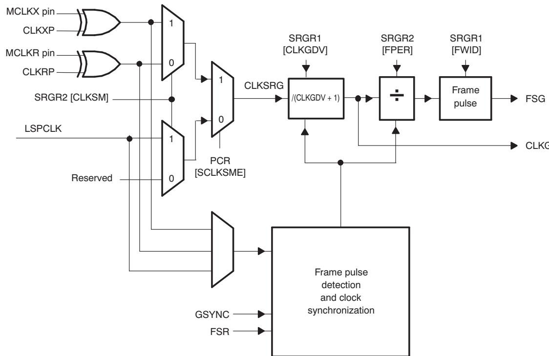
The source clock for the sample rate generator (labeled CLKSRG in the diagram) can be supplied by the LSPCLK, or by an external pin (MCLKX or MCLKR). The source is selected with the SCLKSME bit of PCR and the CLKSM bit of SRGR2. If a pin is used, the polarity of the incoming signal can be inverted with the appropriate polarity bit (CLKXP of PCR or CLKRP of PCR).
