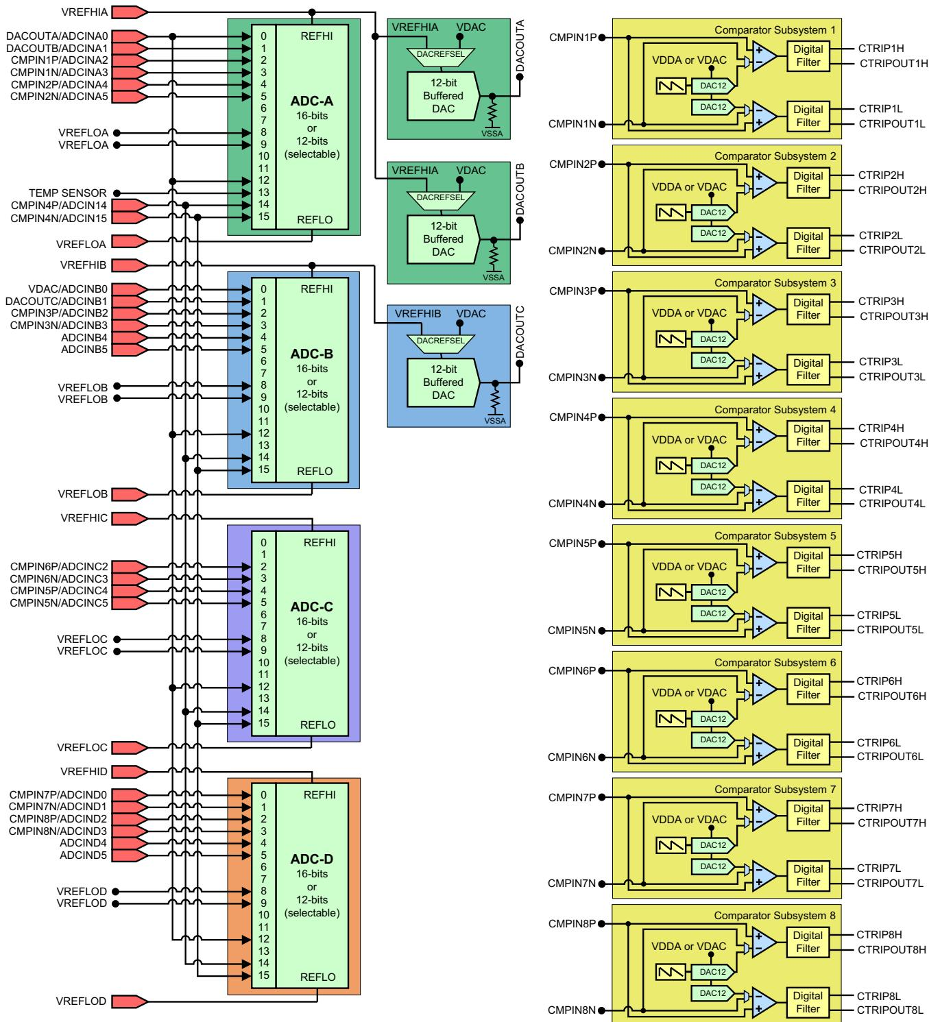
**Figure 9-2. Analog Subsystem Block Diagram (176-Pin PTP)**
