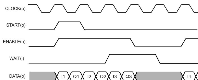
**NOTE:** START asserts on every data word from DMA Channel I in interleaving mode.
