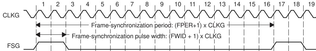
When the sample rate generator comes out of reset, FSG is in its inactive state. Then, when GRST = 1 and FSGM = 1, a frame-synchronization pulse is generated. The frame width value (FWID + 1) is counted down on every CLKG cycle until it reaches 0, at which time FSG goes low. At the same time, the frame period value (FPER + 1) is also counting down. When this value reaches 0, FSG goes high, indicating a new frame.
