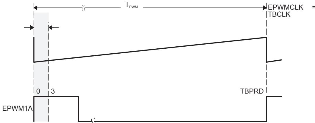
**Table 14-16. Duty Cycle Range Limitation for Three EPWMCLK/TBCLK Cycles**
