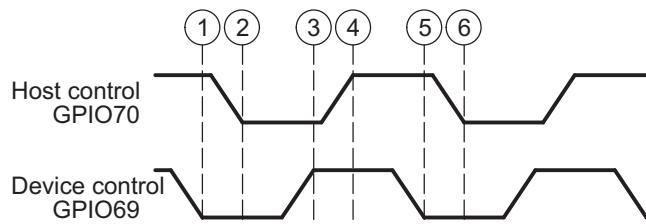
1. The device indicates it is ready to start receiving data by pulling the GPIO69 pin low.
