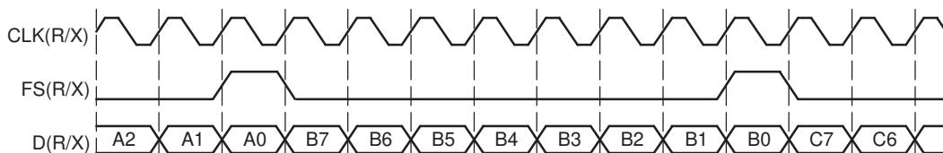
If there is a 1-bit data delay as shown in this figure, the frame-synchronization pulse overlaps the last bit transmitted in the previous frame. Effectively, this permits a continuous stream of data, making frame-synchronization pulses redundant. Theoretically, only an initial frame-synchronization pulse is required to initiate a multipacket transfer.
