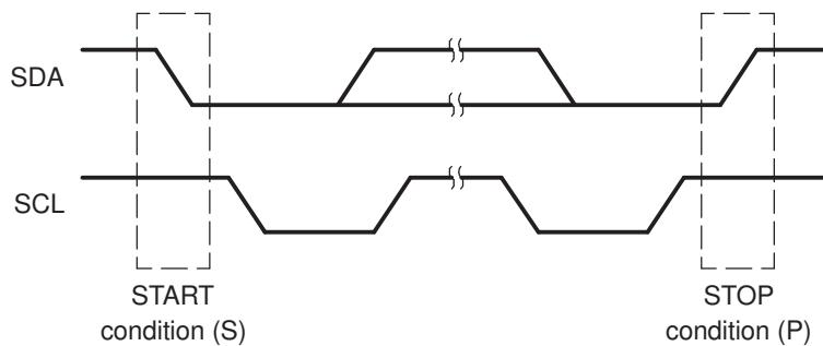
After a START condition and before a subsequent STOP condition, the I2C bus is considered busy, and the bus busy (BB) bit of I2CSTR is 1. Between a STOP condition and the next START condition, the bus is considered free, and BB is 0.
