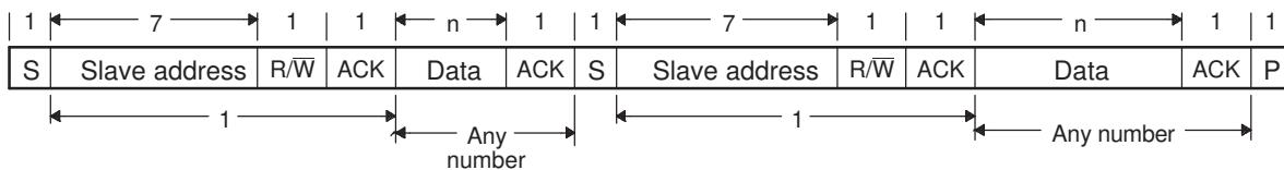
**NOTE:** In [Figure 19-11](#), n = the number of data bits (from 1 to 8) specified by the bit count (BC) field of I2CMDR.
