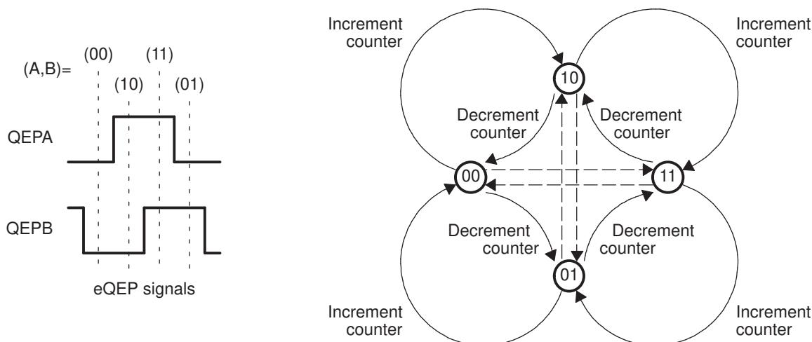
**Figure 16-7. Quadrature-clock and Direction Decoding**
