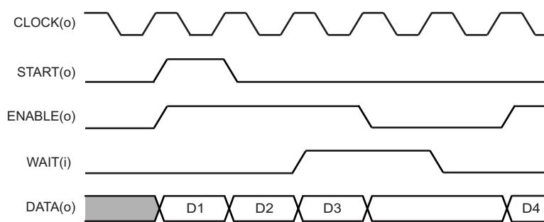
**Figure 23-12. uPP Transmit in SDR Mode – Interleaving**
