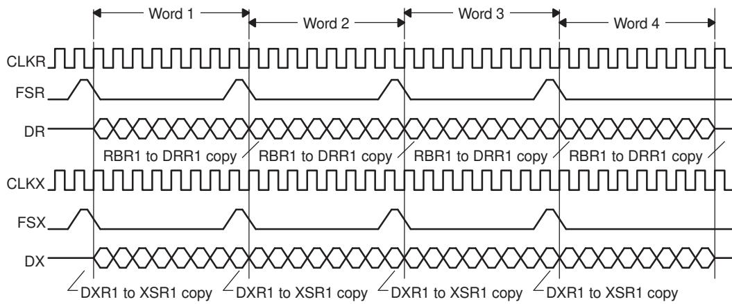
Figure 20-64 shows the McBSP configured to treat this data stream as a continuous 32-bit word. In this example, the McBSP responds to an initial frame-synchronization pulse. However, (R/X)FIG = 1 so that the McBSP ignores subsequent pulses. Only two read transfers or two write transfers are needed every 32 bits. This configuration effectively reduces the required bus bandwidth to half the bandwidth needed to transfer four 8-bit words.
