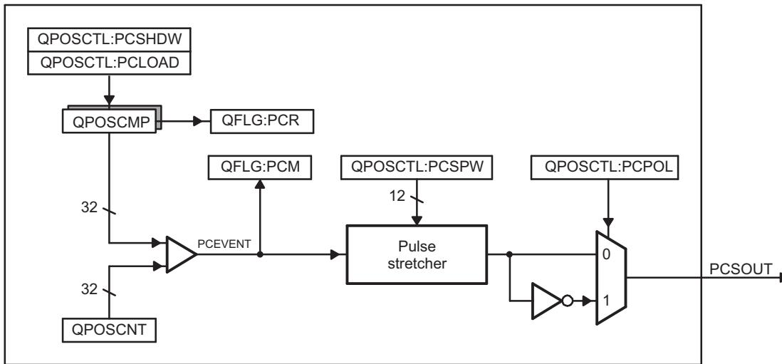
In shadow mode, you can configure the position-compare unit (QPOSCTRL[PCLOAD]) to load the shadow register value into the active register on the following events, and to generate the position-compare ready (QFLG[PCR]) interrupt after loading.
