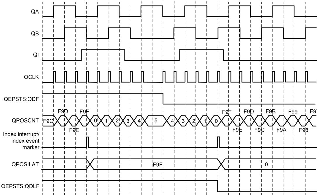
**NOTE:** In case of boundary condition where time period between Index Event and previous QCLK edge is less than SYSCLK period, then QPOSCNT gets reset to zero or QPOSMAX in the same SYSCLK cycle and does not wait for next QCLK edge to occur.
