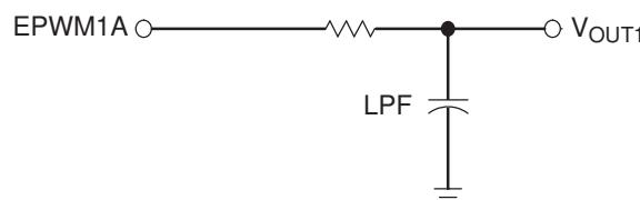
**Figure 14-92. PWM Waveform Generated for the PWM DAC Function**
