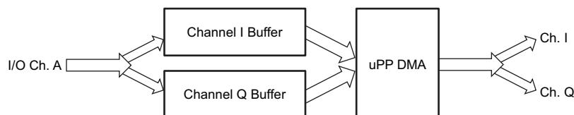
[Figure 23-5](#) explains the data flow for transmit in SDR non-interleave or DDR non-demux mode. In this case, only one DMA channel (channel I) get used.
