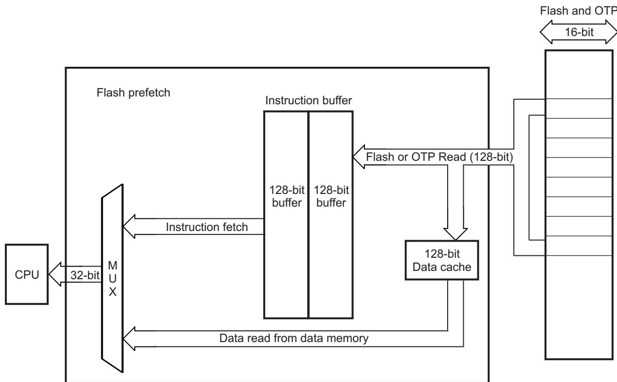
This prefetch mechanism does a look-ahead prefetch on linear address increments starting from the address of the last instruction fetch. The flash prefetch mechanism is disabled by default. Setting the PREFETCH\_EN bit in the FRD\_INTF\_CTRL register enables this prefetch mode.
