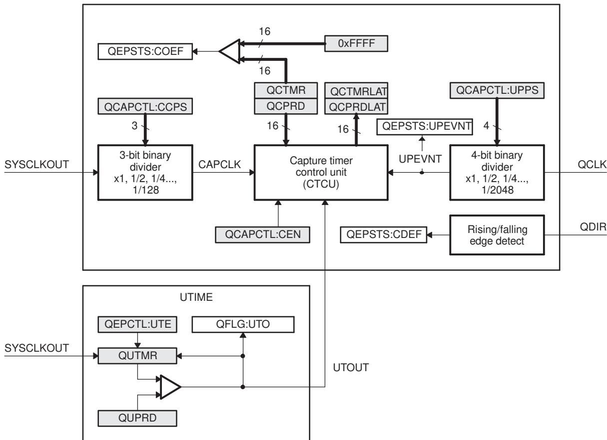
**NOTE:** The QCAPCTL[UPPS] prescaler should not be modified dynamically (such as switching the unit event prescaler from QCLK/4 to QCLK/8). Doing so may result in undefined behavior. The QCAPCTL[CCPS] prescaler can be modified dynamically (such as switching CAPCLK prescaling mode from SYSCLK/4 to SYSCLK/8) only after the capture unit is disabled.
