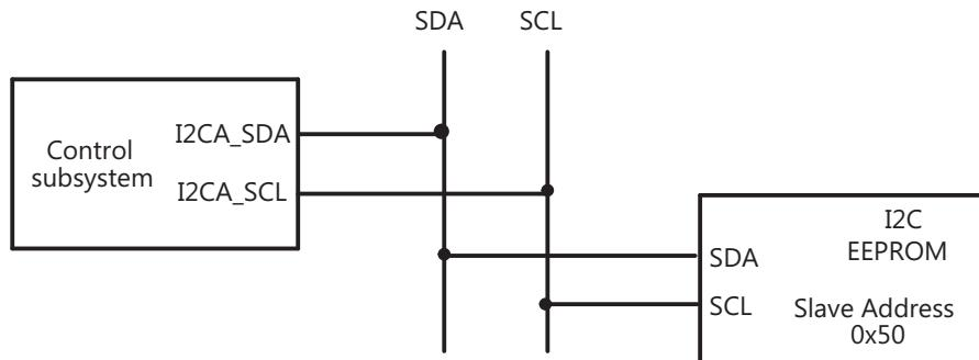
If the download is to be performed from a device other than an EEPROM, then that device must be set up to operate in the slave mode and mimic the I<sup>2</sup>C EEPROM. Immediately after entering the I<sup>2</sup>C boot function, the GPIO pins are configured for I<sup>2</sup>C-A operation and the I<sup>2</sup>C is initialized. The following requirements must be met when booting from the I<sup>2</sup>C module:
