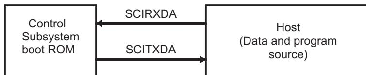
The device communicates with the external host by communication through the SCI-A peripheral. The autobaud feature of the SCI port is used to lock baud rates with the host. For this reason the SCI loader is very flexible and you can use a number of different baud rates to communicate with the device.
