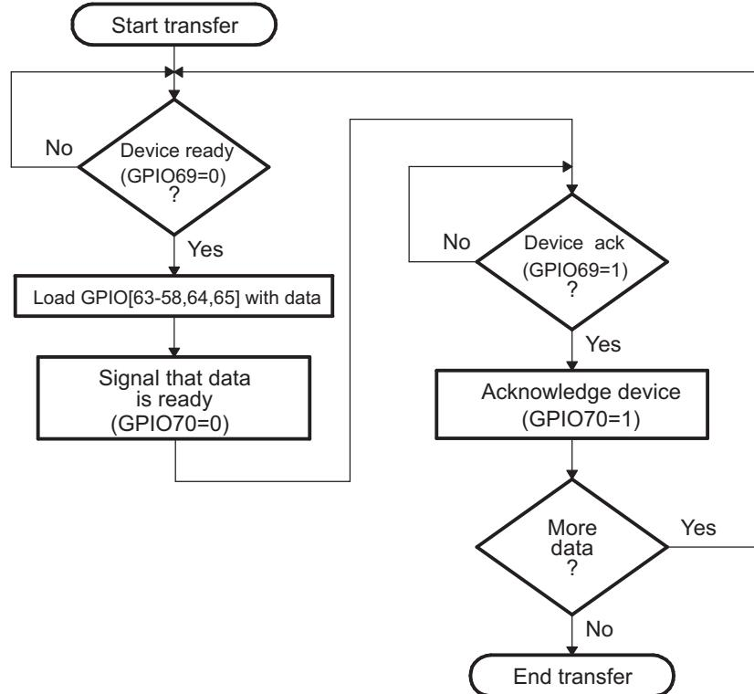
[Figure 4-17](#) shows the flow used to read a single word of data from the parallel port.
