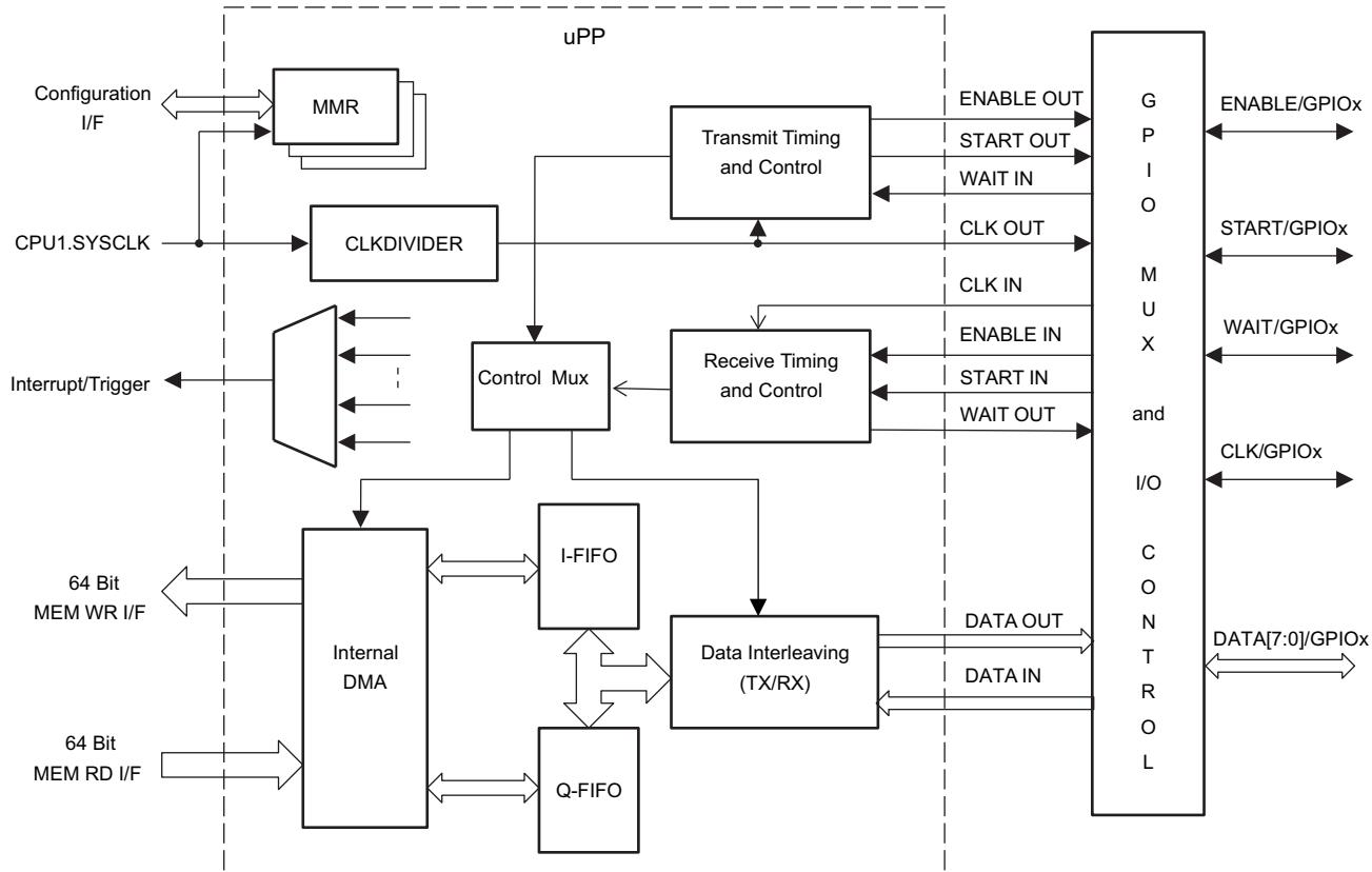
The uPP IP supports internal FIFO to store the data to and from IOs. To alleviate the load of data transfer from system memory to and from the uPP FIFOs, the IP supports internal DMA. The internal DMA has two channels: channel I and channel Q.
