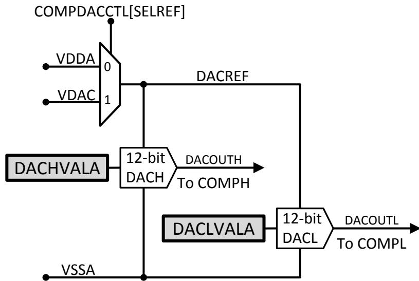
The ideal output of the reference 12-bit DAC can be calculated as follows:
