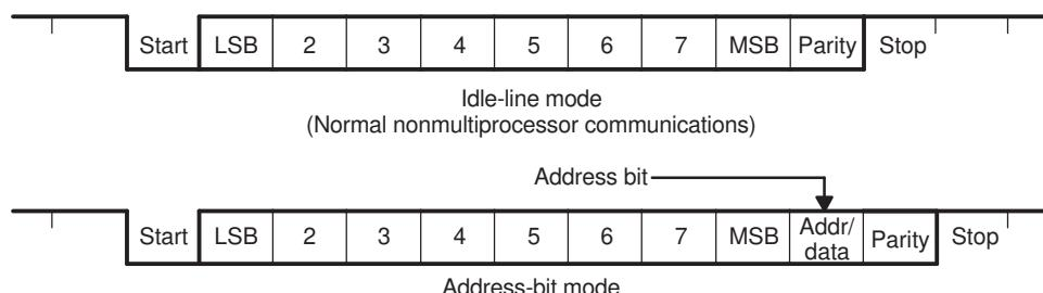
To program the data format, use the SCICCR register. The bits used to program the data format are shown in [Table 18-2](#).
