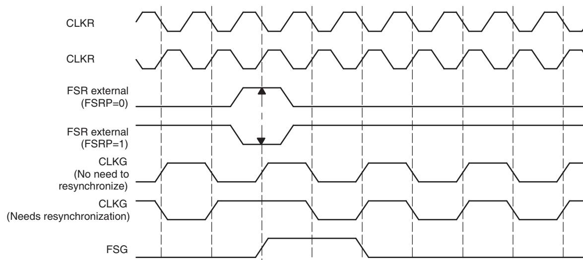
**Figure 20-20. CLKG Synchronization and FSG Generation When GSYNC = 1 and CLKGDV = 3**
