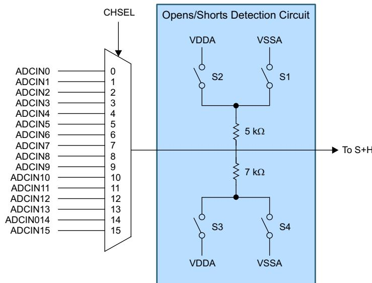
The circuit can be operated by writing a value to the DETECTCFG field in the ADCOSDETECT register. This will cause the circuit to source a voltage onto the input during the S+H phase of any conversion. The voltage and drive strength of the OSDETECT circuit for different DETECTCFG settings is given in Table 10-8.
