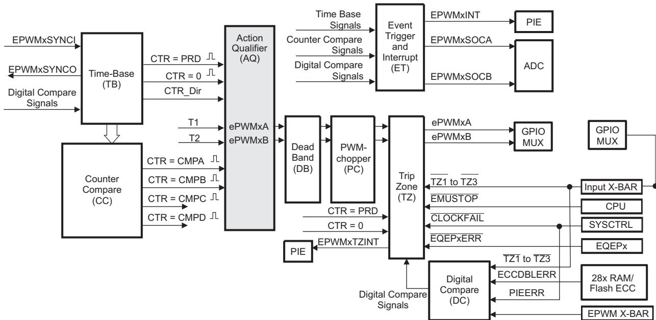
The action-qualifier submodule has the most important role in waveform construction and PWM generation. It decides which events are converted into various action types, thereby producing the required switched waveforms at the EPWMxA and EPWMxB outputs.
