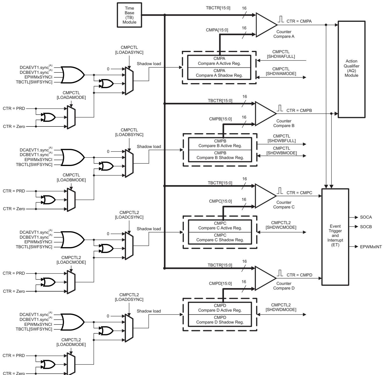
A These events are generated by the type 4 ePWM digital compare (DC) submodule based on the levels of the TRIPIN inputs(for example, CMPSSx and  $\overline{TZ}$  signals).
