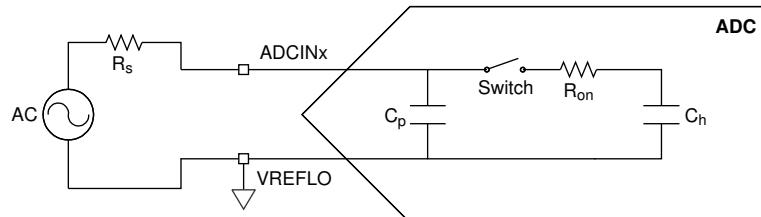
For differential operation, the ADC input characteristics for values in the differential input model (see [Figure 10-4](#)) can be found in the device data manual.
