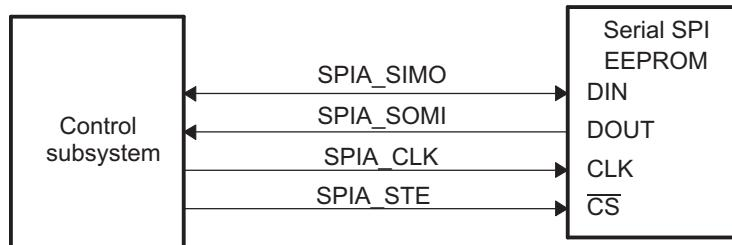
The SPI boot ROM loader initializes the SPI module to interface to a serial SPI EEPROM or flash. Devices of this type include, but are not limited to, the Xicor X25320 (4Kx8) and Xicor X25256 (32Kx8) SPI serial SPI EEPROMs and the Atmel AT25F1024A serial flash.
