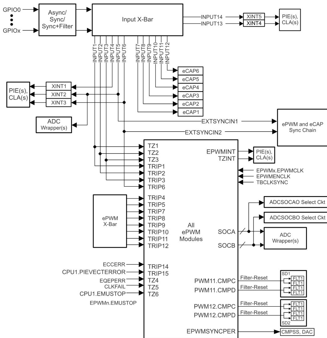
On this device, any of the GPIO pins can be flexibly mapped to be the trip-zone input and/or trip inputs to the trip-zone submodule and digital compare submodule. The Input X-BAR Input Select (INPUTxSELECT) register defines which GPIO pins gets assigned to be the trip-zone inputs / trip inputs.
