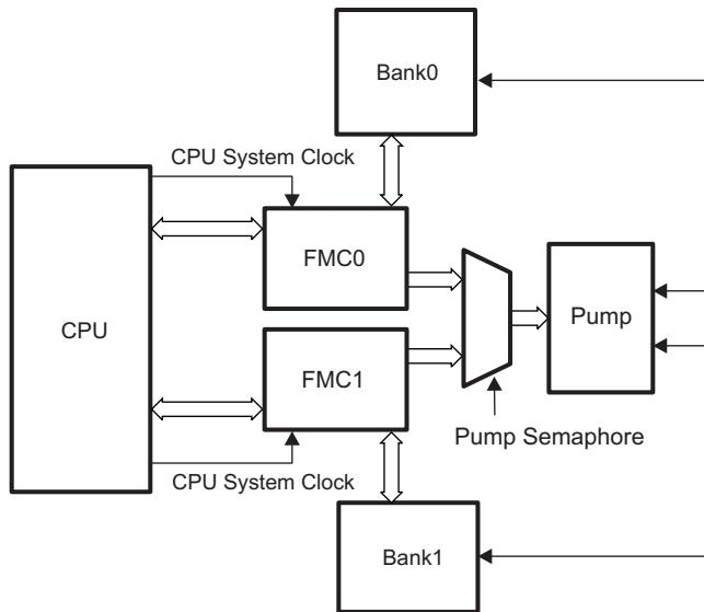
The CPU interfaces with FMC1 which in turn, interfaces with Bank1 and the shared pump to perform erase or program operations as well as to read data and execute code from Bank1. Control signals to the flash pump will be controlled by either FMC0 or FMC1, depending on who gains the flash pump semaphore.
