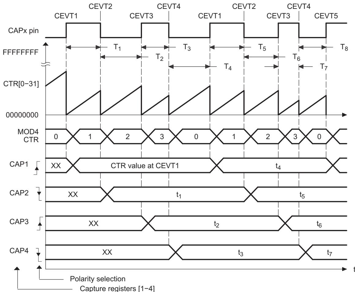
During initialization, you must write to the active registers for both period and compare. This action will automatically copy the init values into the shadow values. For subsequent compare updates during run-time, the shadow registers must be used.
