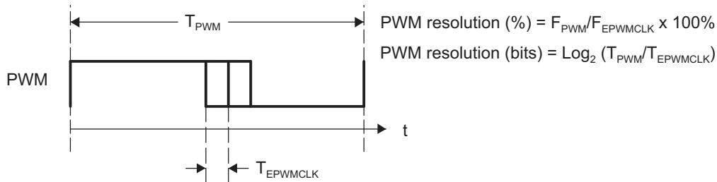
If the required PWM operating frequency does not offer sufficient resolution in PWM mode, you may want to consider HRPWM. As an example of improved performance offered by HRPWM, the table below shows resolution in bits for various PWM frequencies. These values assume a MEP step size of 180 ps. See the device-specific data sheet for typical and maximum performance specifications for the MEP.
