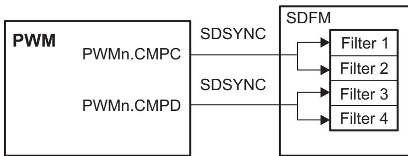
**NOTE:** Ensure that ONLY ONE SDSYNC event will be generated per PWM timer period. Using PWM in up-count or down-count mode would automatically ensure that you get ONLY SDSYNC event. But, if up-down count mode is used, then make sure that only one SDSYNC event per PWM cycle is generated; otherwise, the filter synchronizer will corrupt SDFM timing by providing two pulses per PWM cycle.
