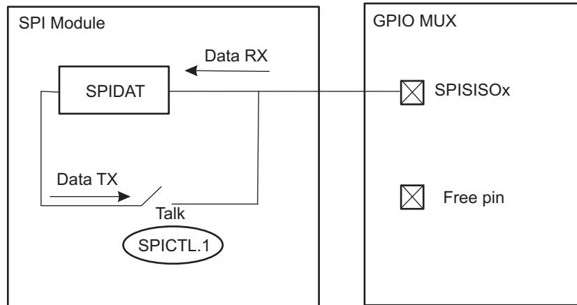
**Table 17-5** indicates how data is received or transmitted in the various SPI modes while the TALK bit is set or cleared.
