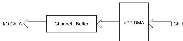
[Figure 23-6](#) explains the data flow for transmit in SDR interleave or DDR demux mode. In this case, both DMA channels (channel I and channel Q) are used.
