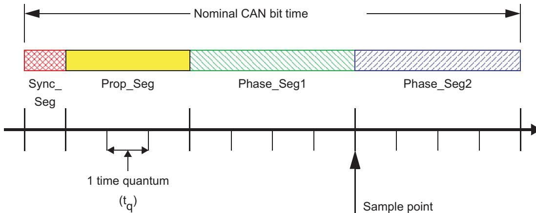
Each segment consists of a specific number of time quanta. The length of one time quantum ( $t_q$ ), which is the basic time unit of the bit time, is given by the CAN\_CLK and the Baud Rate Prescalers (BRPE and BRP). With these two Baud Rate Prescalers combined, divider values from 1 to 1024 can be programmed:
