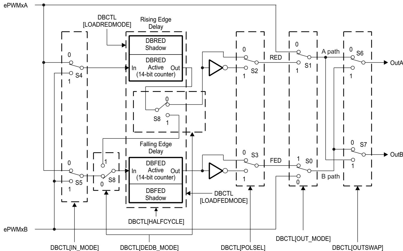
Although all combinations are supported, not all are typical usage modes. [Table 14-8](#) documents some classical dead-band configurations. These modes assume that the DBCTL[IN\_MODE] is configured such that EPWMxA In is the source for both falling-edge and rising-edge delay. Enhanced, or non-traditional modes can be achieved by changing the input signal source. The modes shown in [Table 14-8](#) fall into the following categories:
