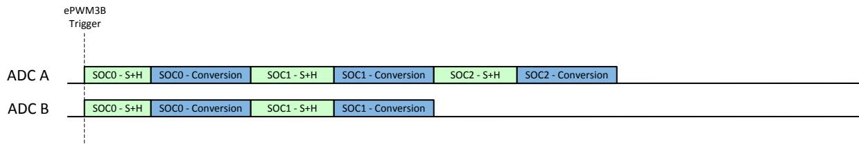
Note that if the trigger comes again before all SOCs have completed their conversions, ADCB will begin converting immediately on SOC0 while ADCA will not start converting SOC0 again until SOC2 is complete. This will result in asynchronous operation, so care must be taken to not overflow the trigger.
