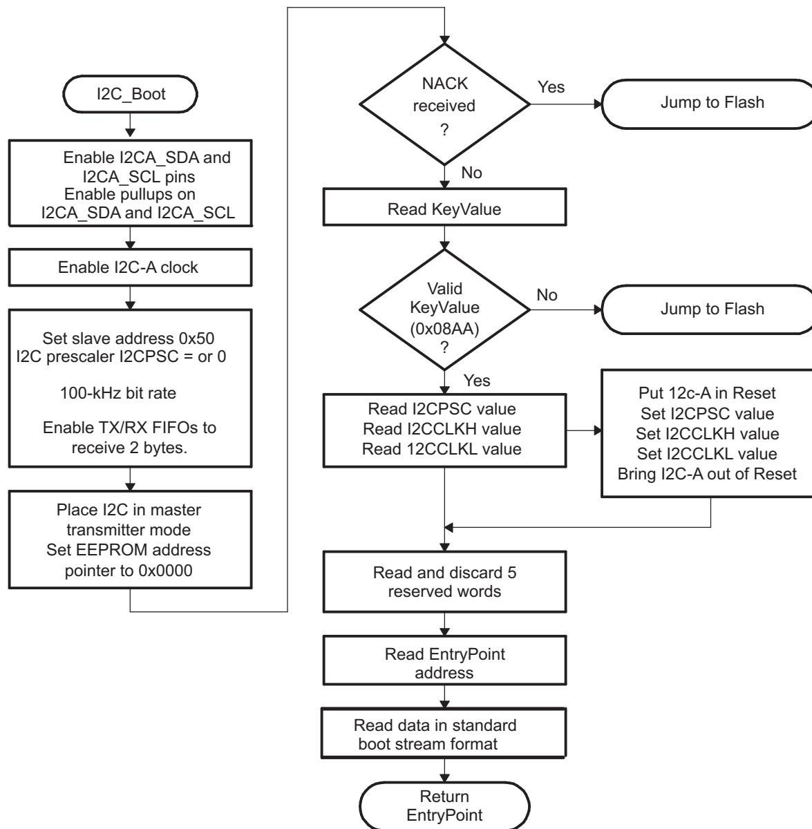
The bit-period prescalers (I<sub>2</sub>CCLKH and I<sub>2</sub>CCLKL) are configured by the bootloader to run the I<sub>2</sub>C at a 50 percent duty cycle at 100-kHz bit rate (standard I<sub>2</sub>C mode) when the system clock is 10 MHz. These registers can be modified after receiving the first few bytes from the EEPROM. This allows the communication to be increased up to a 400-kHz bit rate (fast I<sub>2</sub>C mode) during the remaining data reads.
