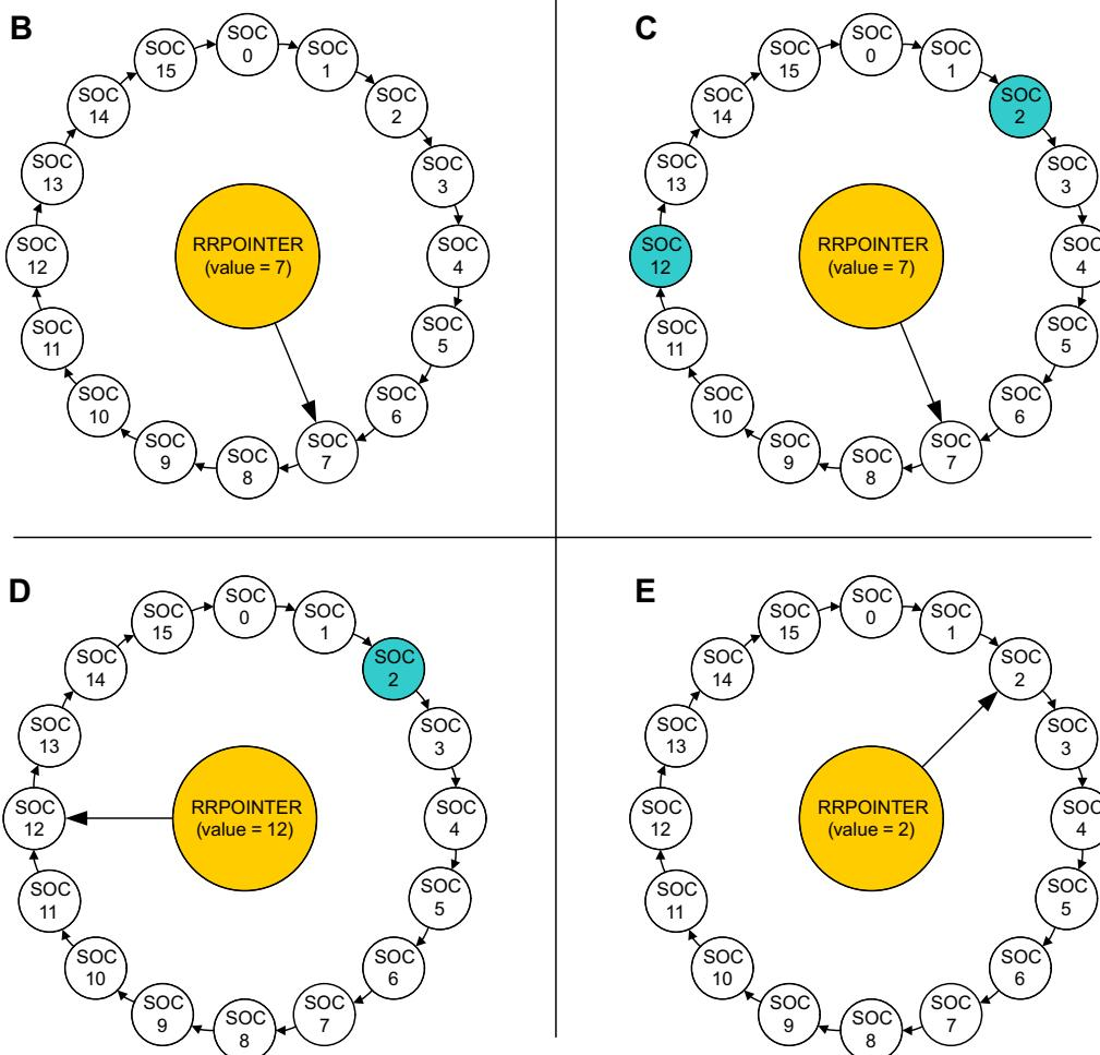
The SOC\_PRIORITY field in the ADCSOC\_PRIORITYCTL register can be used to assign high priority from a single to all of the SOCs. When configured as high priority, an SOC will interrupt the round robin wheel after any current conversion completes and insert itself in as the next conversion. After its conversion completes, the round robin wheel will continue where it was interrupted. If two high priority SOC's are triggered at the same time, the SOC with the lower number will take precedence.
