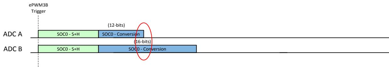
In order to achieve synchronous operation while using both 12-bit and 16-bit resolution, conversions must be done in parallel at one resolution. Once conversions are complete at one resolution, the CPU must switch the resolution on all ADCs and then cause another trigger (this trigger should not be a software SOC force, as all ADCs can't be started simultaneously via this method).
