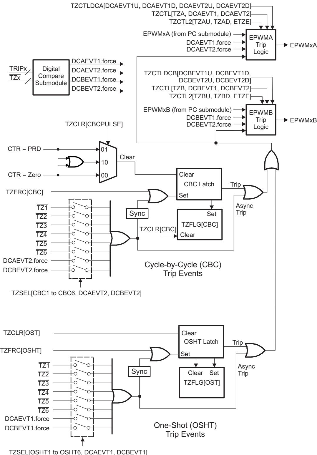
Figure 14-42. Trip-Zone Submodule Interrupt Logic
