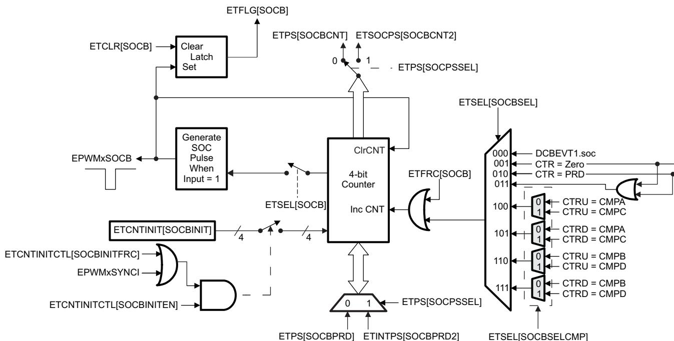
A The DCBEVT1.soc signals are signals generated by the Digital compare (DC) submodule in [Section 14.11](#).
