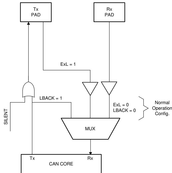
For all test modes, the Test bit in the CAN Control register needs to be set to 1 to enable write access to the CAN\_TEST register.
