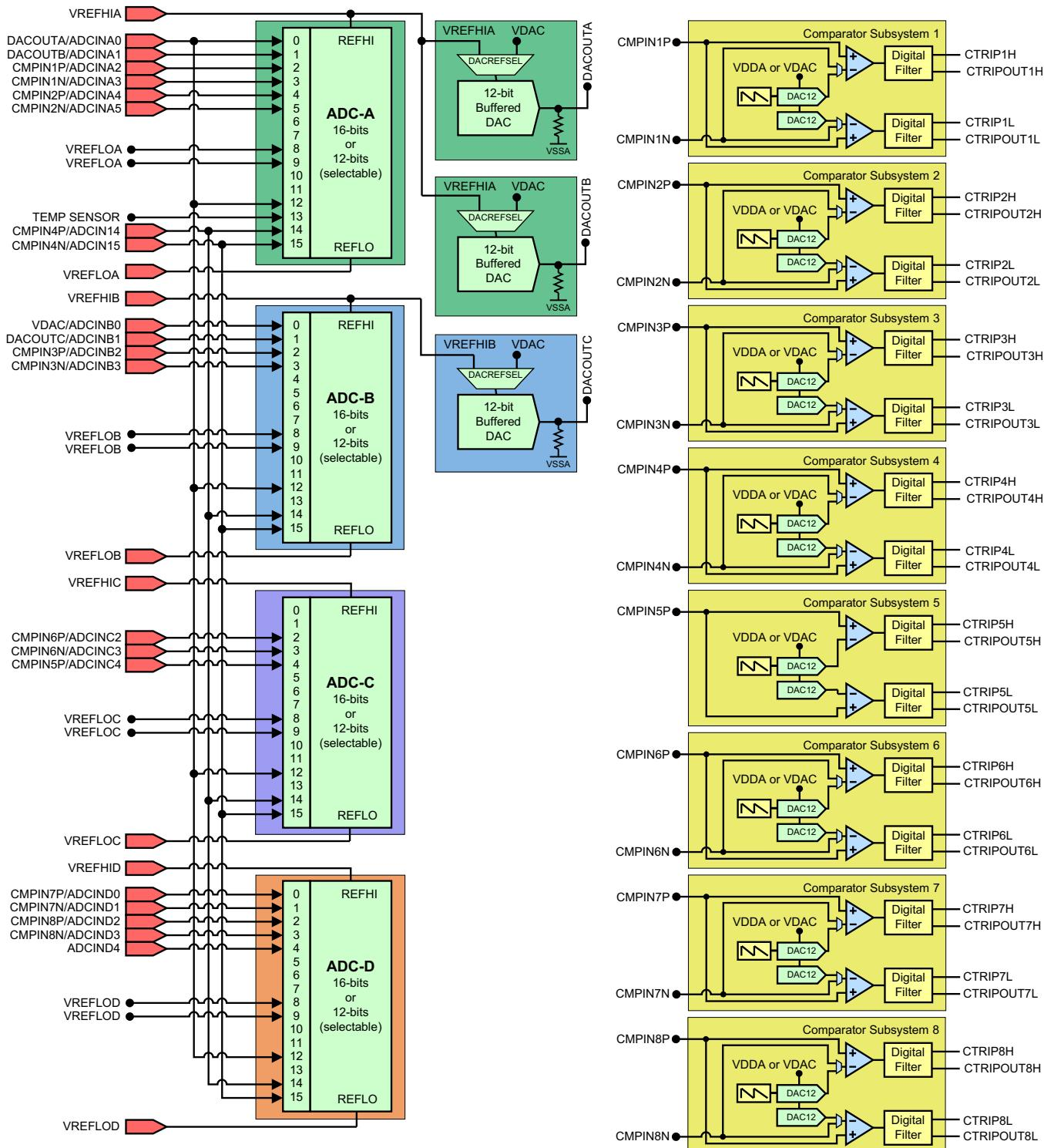
Figure 9-3. Analog Subsystem Block Diagram (100-Pin PZP)
