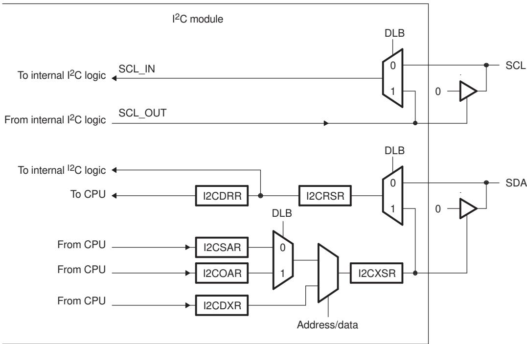
**NOTE:** The free data format (I2CMDR.FDF = 1) is not supported in digital loopback mode.
