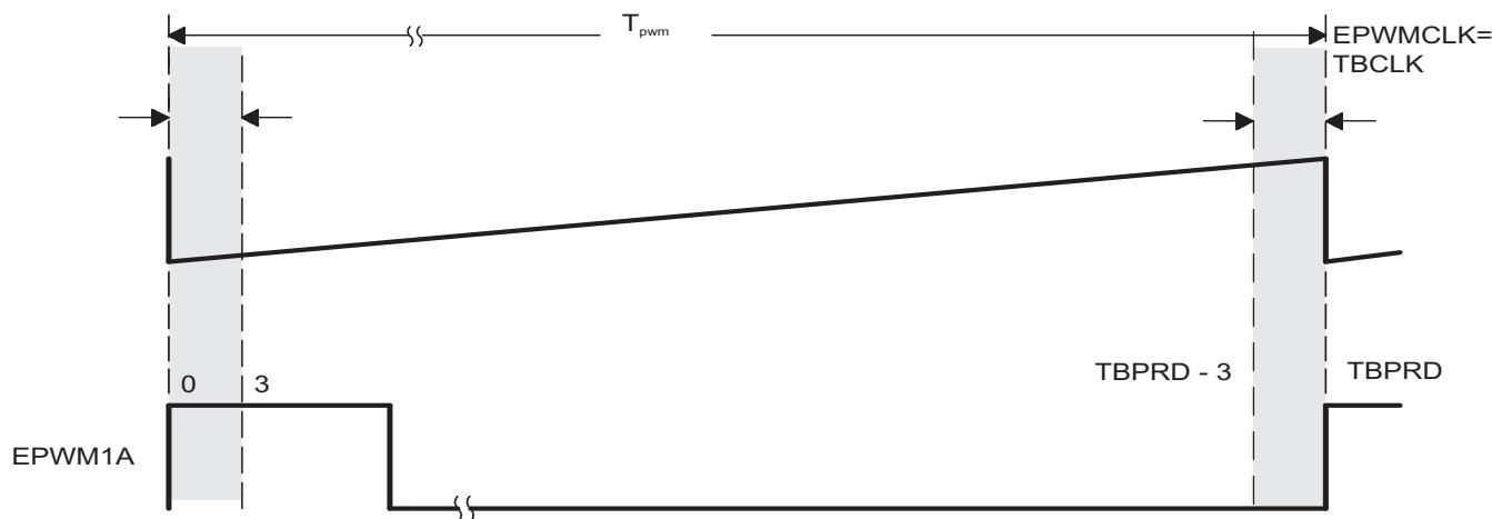
**Figure 14-88. Up-Down Count Duty Cycle Range Limitation Example (HRPCTL[HRPE]=1)**
