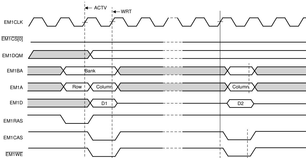
Several other pins are also active during a read access. The EM1DQM[x:0] pins are driven low during the READ commands and are kept low during the NOP commands that correspond to the burst request. The state of the other EMIF pins during each command can be found in [Table 24-6](#).
