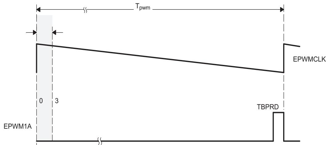
**Figure 14-87. Up-Count Duty Cycle Range Limitation Example (HRPCTL[HRPE]=1)**
