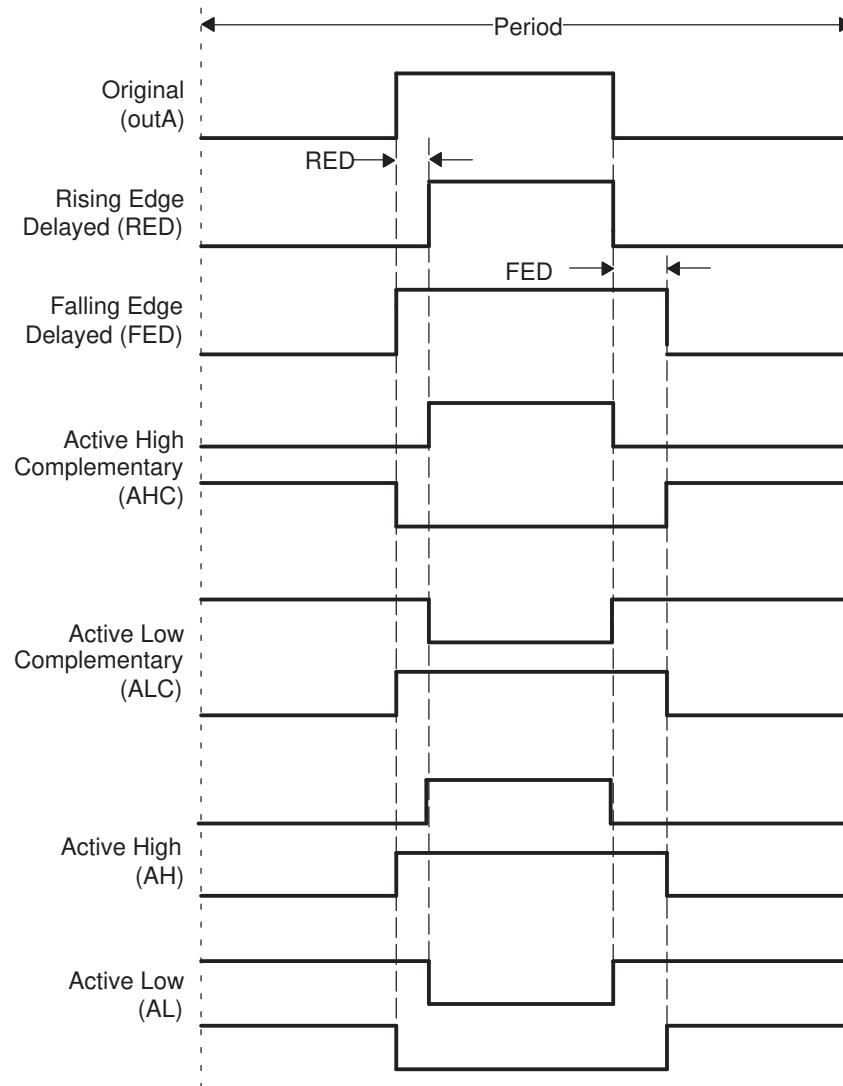
The dead-band submodule supports independent values for rising-edge (RED) and falling-edge (FED) delays. The amount of delay is programmed using the DBRED and DBFED registers. These are 10-bit registers and their value represents the number of time-base clock, TBCLK, periods by which a signal edge is delayed. For example, the formula to calculate falling-edge-delay and rising-edge-delay is:
