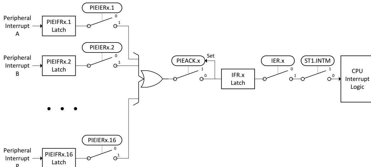
When a peripheral generates an interrupt (on PIE group x, channel y), it triggers the following sequence of events:
