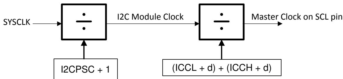
To specify the divide-down value, initialize the IPSC field of the prescaler register, I2CPSC. The resulting frequency is:
