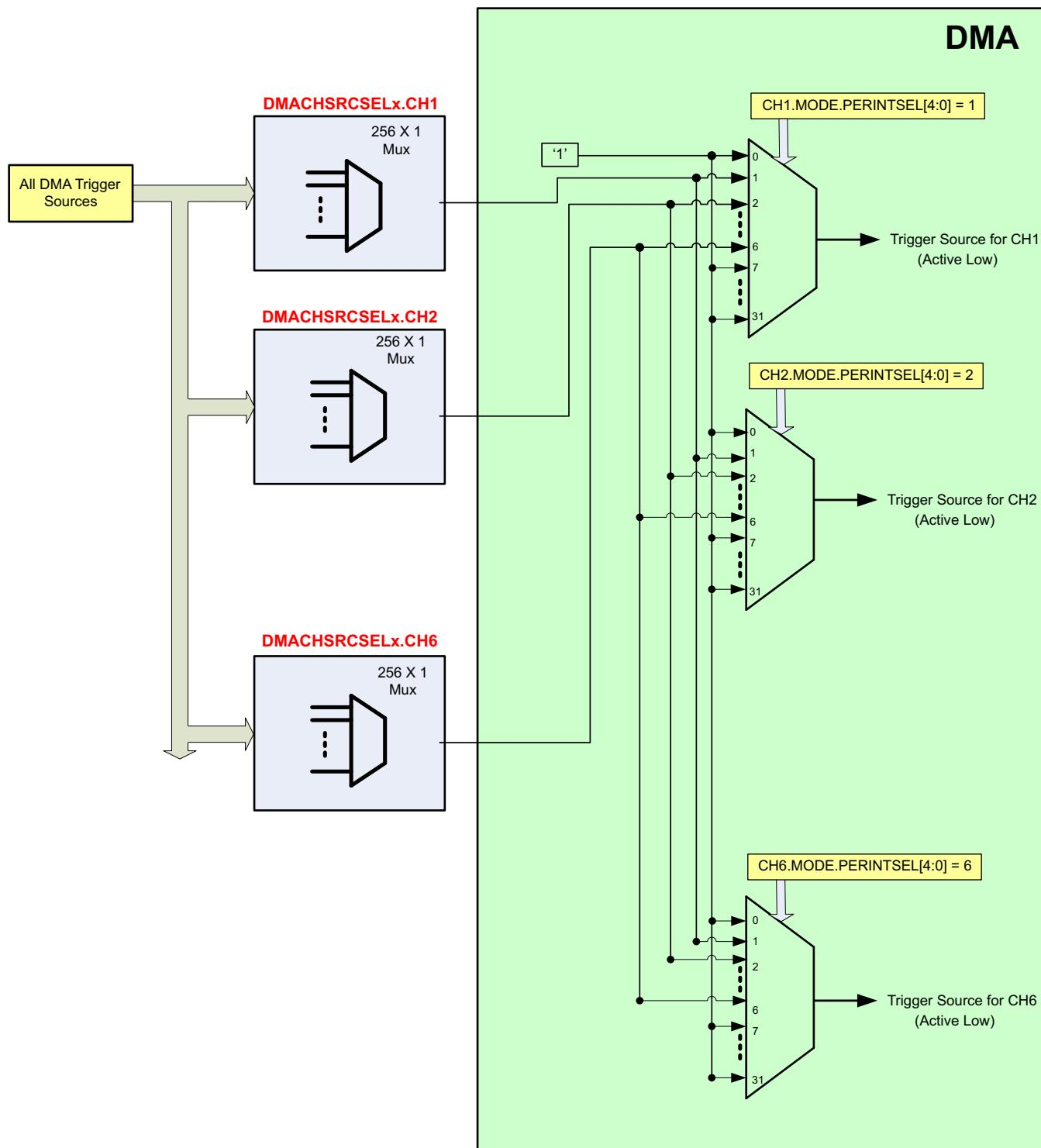
**NOTE:** To use the system level DMA Trigger source selection, the DMA internal trigger source selection configuration for each channel should be done using the DMACHSRCSELx register, and the CH*x*.MODE.PERINTSEL register as shown here. See [Table 5-1](#) or the DMACHSRCSELx register definition for a complete list of DMA trigger sources.
