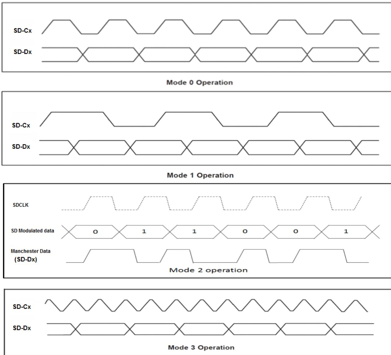
When MOD=2, data and modulated clock signals are encoded into modulated data as shown in Mode 2 of [Figure 13-4](#). In this mode, the clock input SD-Cx pin should be left floating. The input control unit performs continuous automatic calibration to achieve optimum decoding performance.
