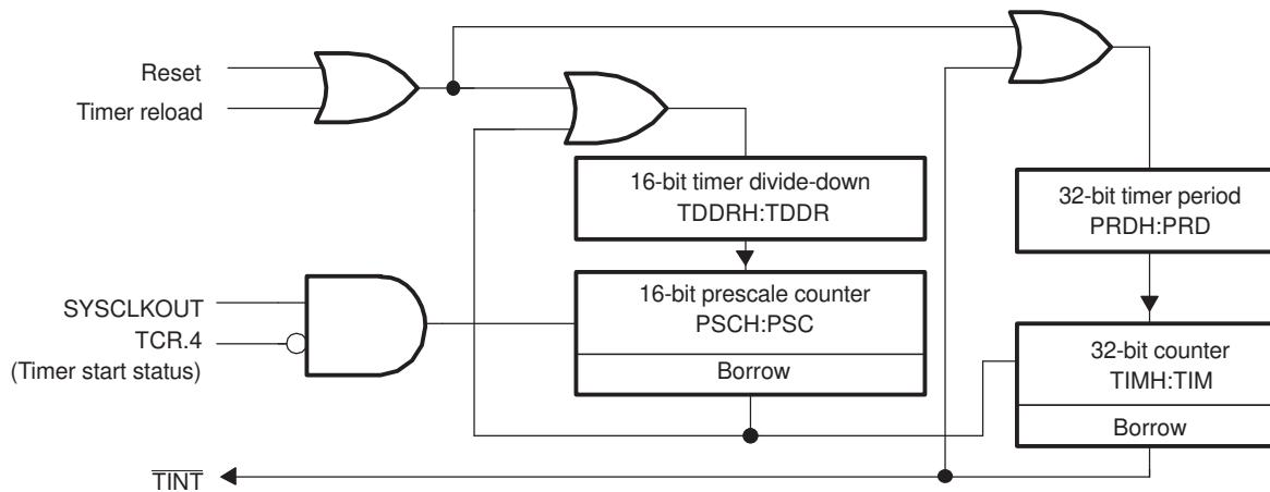
**Figure 3-11. CPU-Timer Interrupts Signals and Output Signal**
