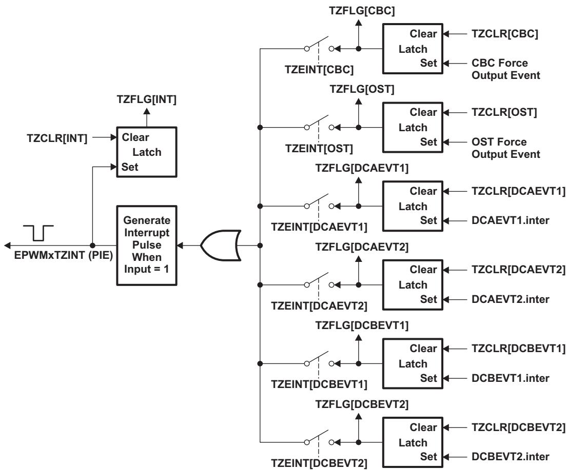
These individual flags for the CBC, OST and DCxEVTy can be used to detect the source of the EPWMxTZINT Interrupt. When multiple sources are used to generate the EPWMxTZINT interrupt, reading and clearing the flags will user to take different actions based on the specific event.
