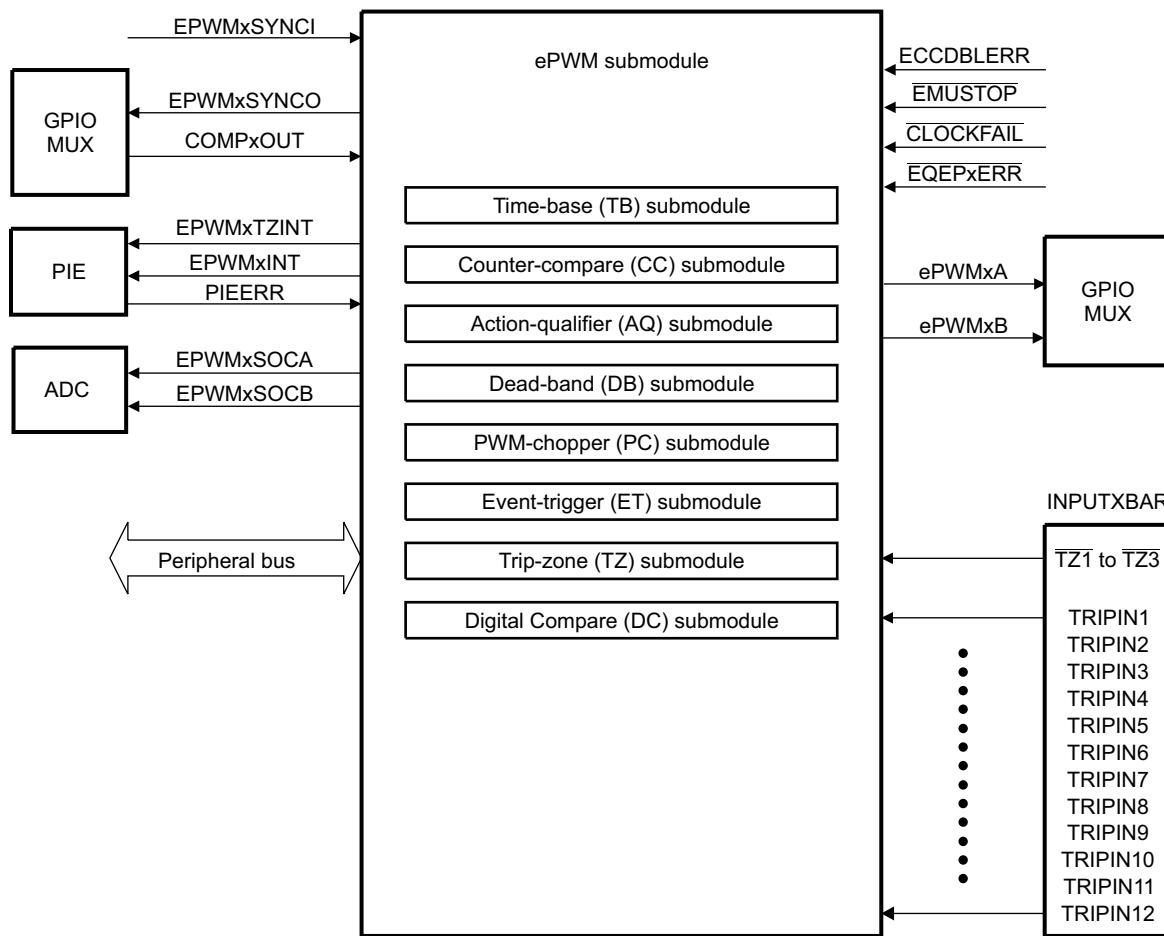
Figure 14-3 shows more internal details of a single ePWM module. The main signals used by the ePWM module are:
