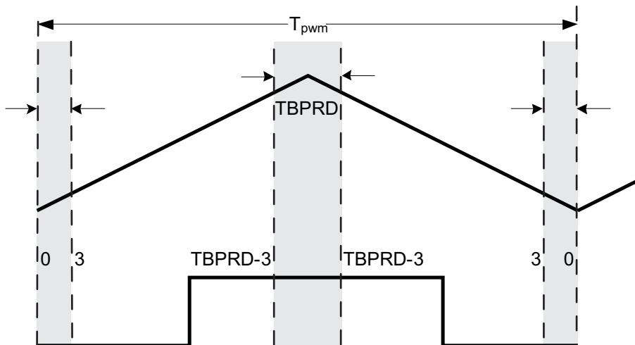
**NOTE:** If the application has enabled high-resolution period control (HRPCTL[HRPE]=1), the duty cycle must not fall within the restricted range. Otherwise, there will be undefined behavior on the ePWM output.
