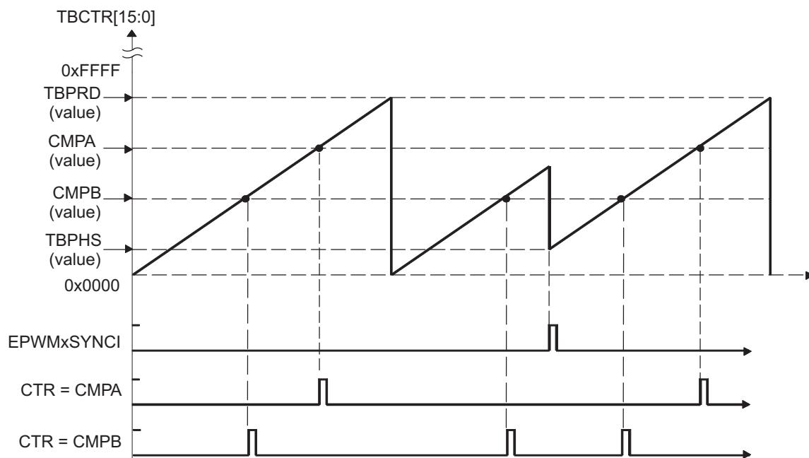
**NOTE:** An EPWMxSYNCI external synchronization event can cause a discontinuity in the TBCTR count sequence. This can lead to a compare event being skipped. This skipping is considered normal operation and must be taken into account.
