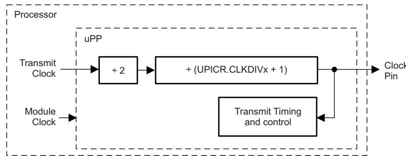
$$\text{Output Clock} = \text{Module Clock} / (2 \times (\text{CLKDIVn} + 1))$$
