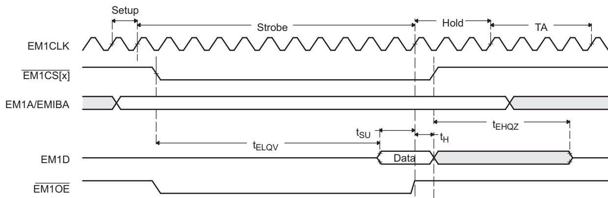
**Figure 24-21. LH28F800BJE-PTTL90 to EMIF Write Timing Waveforms**
