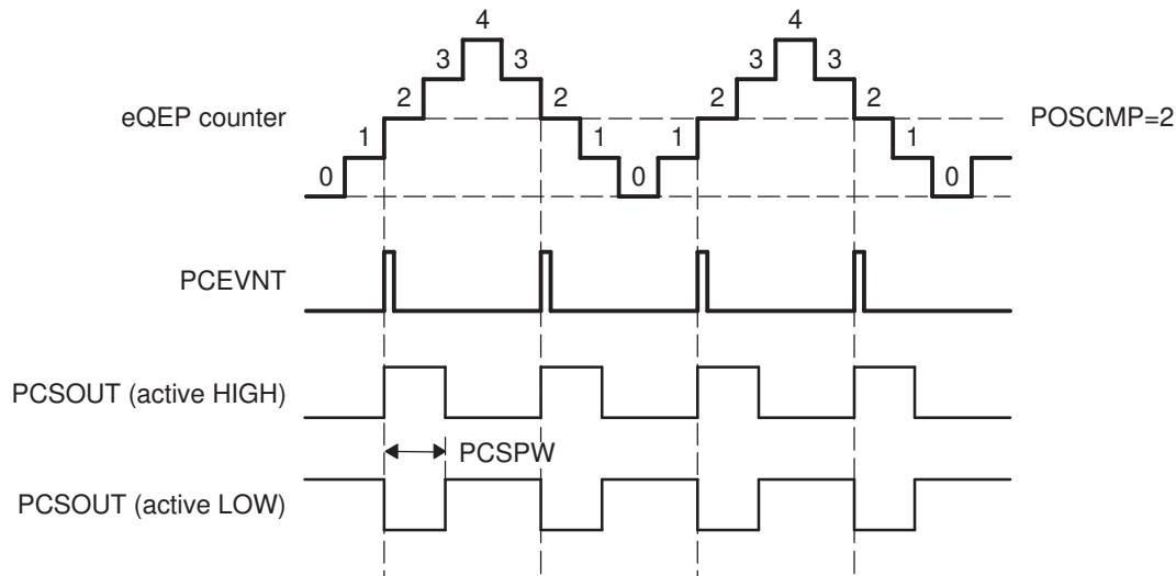
The pulse stretcher logic in the position-compare unit generates a programmable position-compare sync pulse output on the position-compare match. In the event of a new position-compare match while a previous position-compare pulse is still active, then the pulse stretcher generates a pulse of specified duration from the new position-compare event as shown in [Figure 16-14](#).
