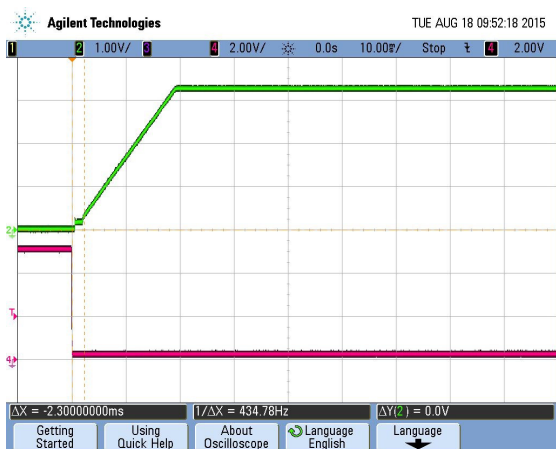
Enable Startup Delay (Vin = 48V, Iout = 60A, Cloud = 1000uF, Ta = +25°C) Ch2 = Vout, Ch4 = Enable
