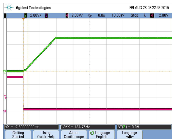
Enable Startup Delay (Vin = 48V, Iout = 60A, Cload = 1000uF, Ta = +25°C) Ch2 = Vout, Ch4 = Enable
