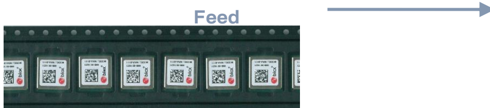
Figure 13: Orientation of NINA-W151 module on tape
