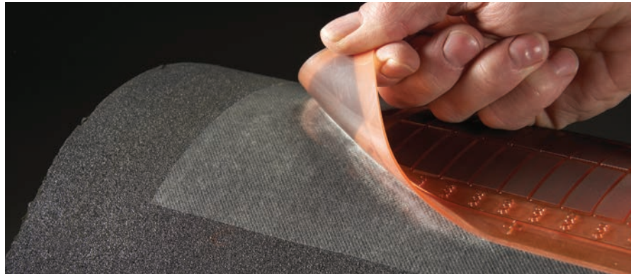
3M™ Thin Flexographic Plate Mounting Tape E2105 is a double coated film tape constructed of a polyester film carrier with differential adhesives specifically designed for mounting flexographic print plates to cushioned/compressible sleeves.
