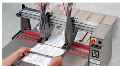
Automatic and semi-automatic equipment is available for higher volume applications. For example, apply tape to business forms, literature, bounce back and business reply cards.
