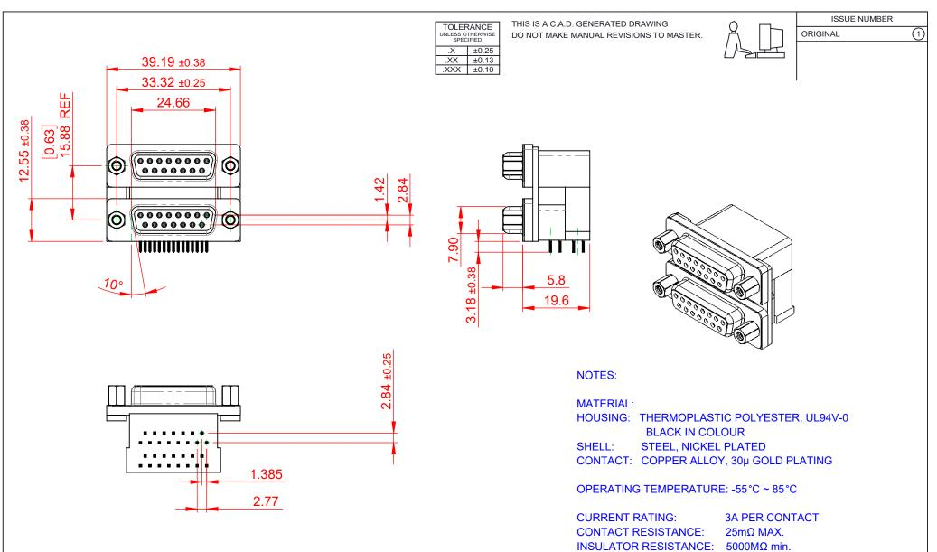
DIELECTRIC WITHSTANDING VOLTAGE: 1000V AC rms
