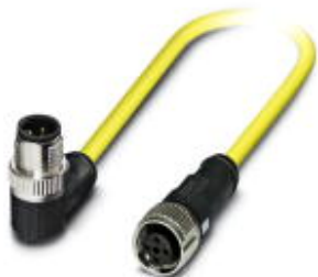
Sensor/actuator cable, 4-position, PVC, yellow, Plug angled M12 SPEEDCON, A-coded, on Socket straight M12 SPEEDCON, A-coded, cable length: 0.5 m
