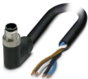
Power cable, 4-position, PVC, black-gray RAL 7021, Plug angled M12, L-coded, on free cable end, cable length: 5 m, for direct current up to 16 A/63 V
