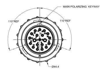
PLUG,18-20 POS,SOCKET CONT.,STANDARD DIA. SEAL, AHDP
