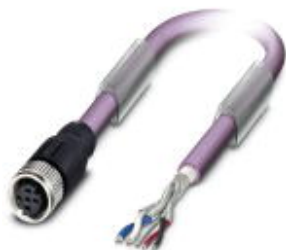
Bus system cable, CANopen®, DeviceNet™, 5-position, PVC, black, shielded, free cable end, on Socket straight M12, A-coded, cable length: 10 m
