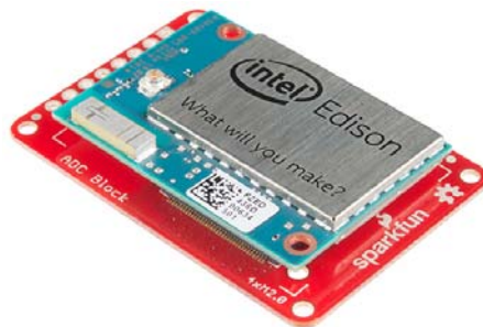
ADC Block Installed
